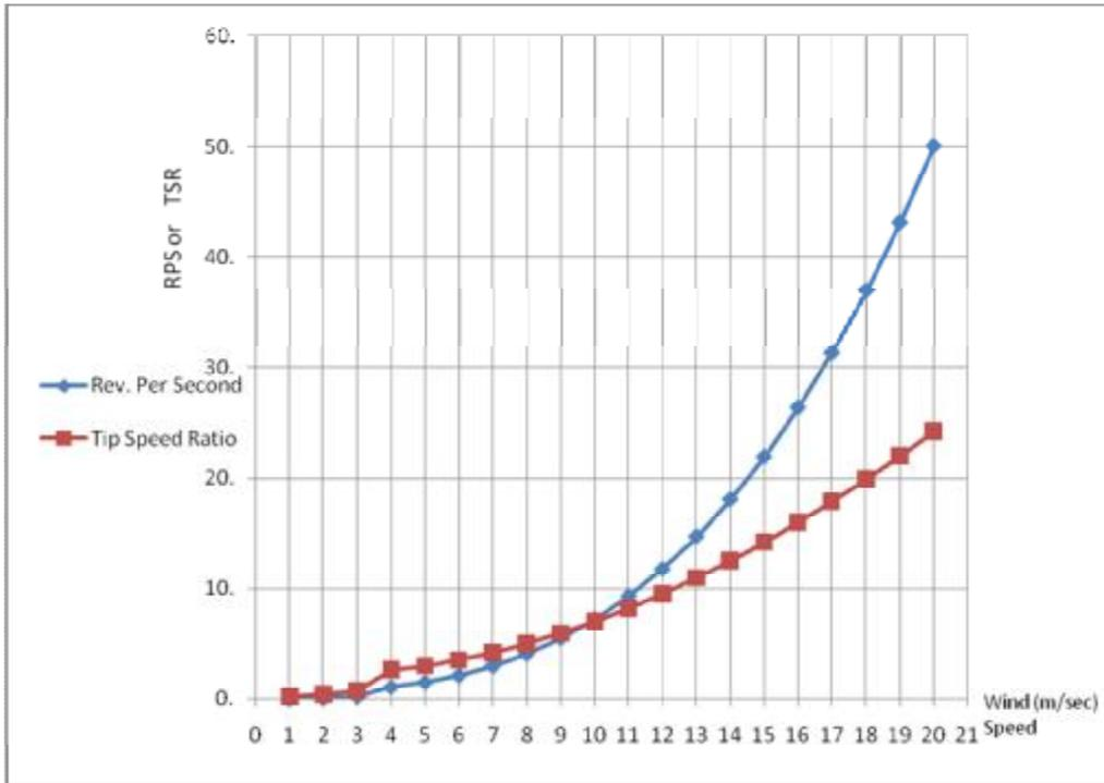
Figure (7): Max. Tip Speed Ratio and Max. Revolution Per Second at any Wind Speed.
