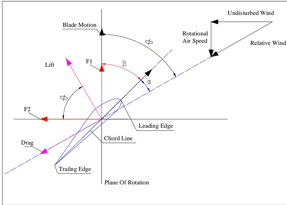
Figure (1):Definitions of pitch angle  $\beta$ , angle of attack  $\alpha$  and all forces and velocities on a translating airfoil.
