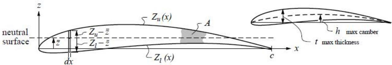
Figure(2): Quantities for determining and estimating the inertia of an airfoil section [10].
