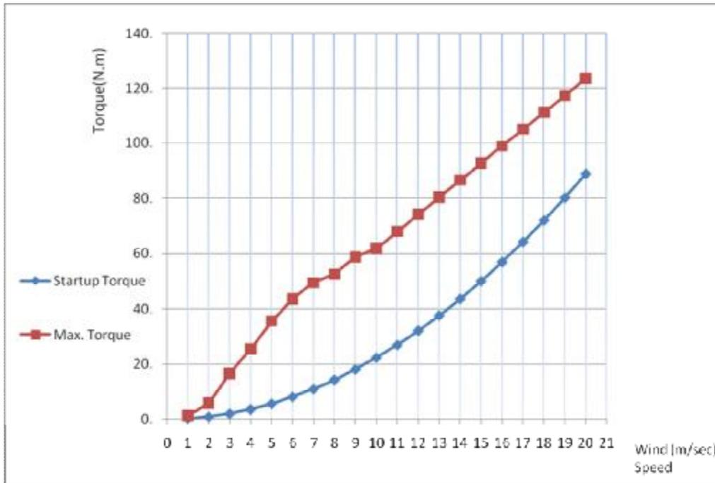
Figure (5): Max. Torque Load and Startup Torque at any Wind Speed.
