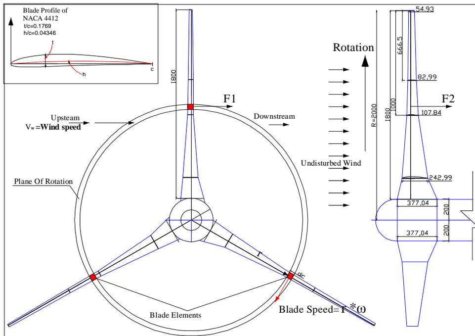
Figure ( 3 ):The wind turbine blades with incoming wind speed and effective forces .
