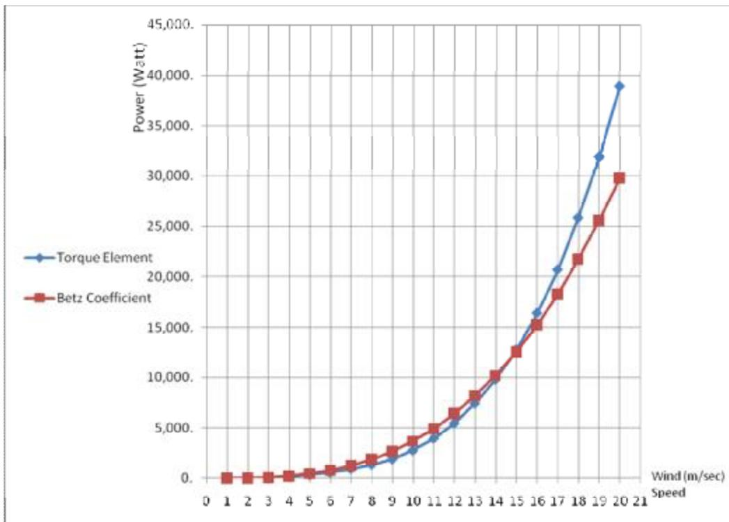
Figure (6): Max. Power Produce by torque element compare with Betz coefficient Theorem at any Wind Speed.
