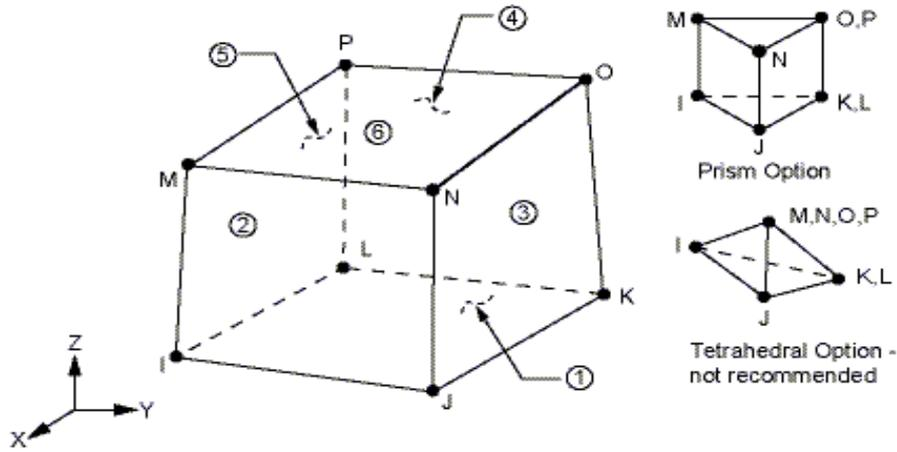
Figure (5) Structural solid geometry of element Solid185[13].
