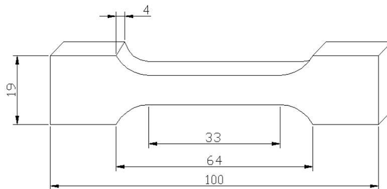
**Figure (1) Standard tensile test specimen (ASTM D412 ) [11]**
