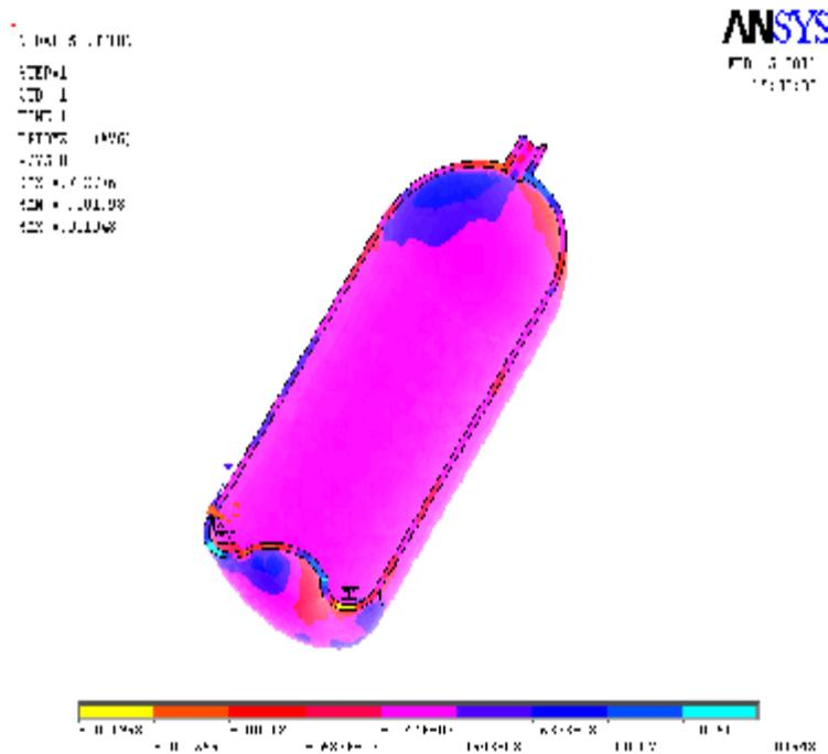
Figure (14) yz- Shear strain analysis of fiber glass orientation with 45 degree at pressure 5 N/mm<sup>2</sup>
