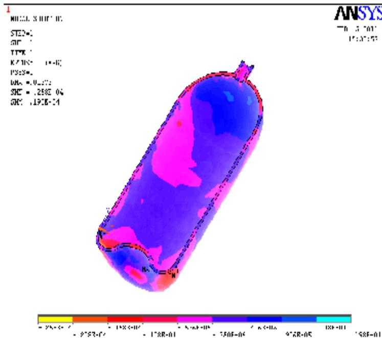
Figure (12) xy- Shear strain analysis of fiber glass orientation with 45 degree at pressure 0.9 N/mm<sup>2</sup>
