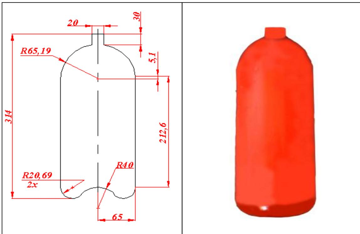
Figure (4) Drawing and Photo of standard fire extinguisher made from metal
