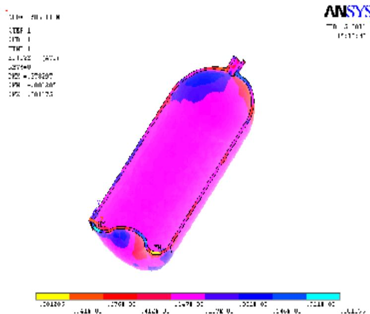
Figure (10) yz- Shear strain analysis of random fiber glass at pressure 5 N/mm<sup>2</sup>
