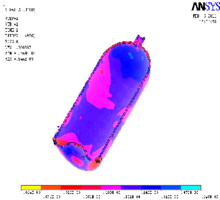
Figure (13) xy- Shear strain analysis of fiber glass orientation with 45 degree at pressure 5 N/mm<sup>2</sup>
