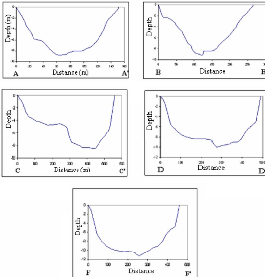
Figure 2. Transverse River Profiles (TRPs) of Shatt Al-Arab River (A-A'): Qurna Section, (B-B'): Nahr Umr Section, (D-D'): Umm Al-Rusas Section, (E-E'): Sihan Section, after MSC, 2005 and (F-F'): Fao Section, after Al-Manssory, 1996.
