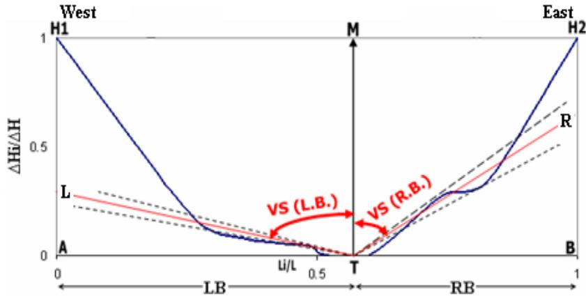
Figure 5. Method of computation of basin symmetry (Bs) and valley (channel) symmetry (Va). Dotted lines are form surfaces of profile curves origination from T (Thalweg of the main river). The angles between the bisectors of the form surface angles at T and the line TM give the actual gradient but  $\angle LTM - \angle RTM$  gives the valley symmetry (Va) and  $AT - 0.5$  gives the basin symmetry (Bs). LB = Left bank; RB = Right bank.
