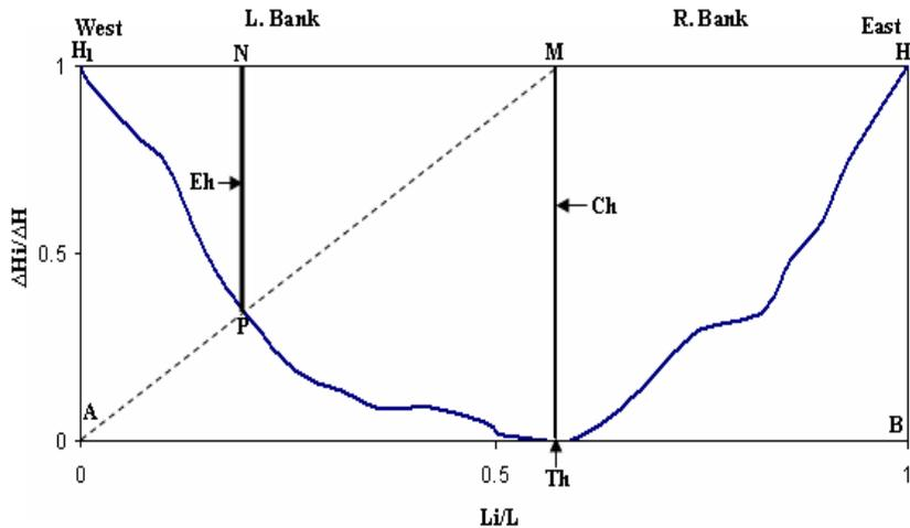
Figure 4. Smoothened hypothetical TRP curve from which  $E_h$  and  $C_h$  are extracted from one channel side. Thalweg  $Th$ . of the main river. For explanation see the text.
