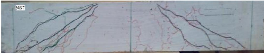
Figure (10) crack pattern and failure mode of beam NS7
