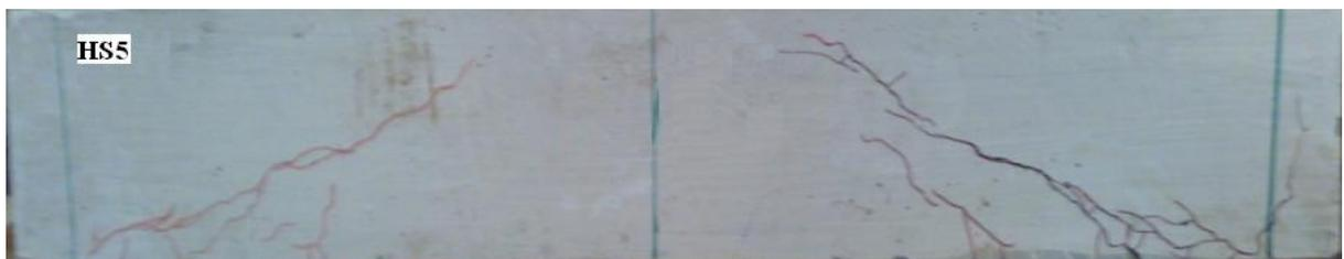
Figure (9) crack pattern and failure mode of beam HS5
