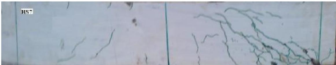
Figure (11) crack pattern and failure mode of beam NS7
