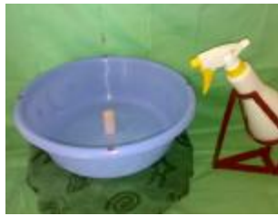
Figure 3: spraying procedure was performed at a fixed distance and fixed angle
