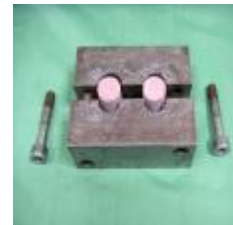
Figure 1: Special split brass mold for preparation of compressive strength and surface roughness test specimens.
