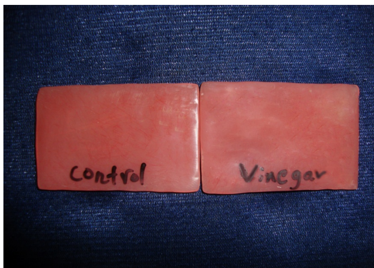
Figure 3: Photographs of specimens Immersed in distilled water and Vinegar
