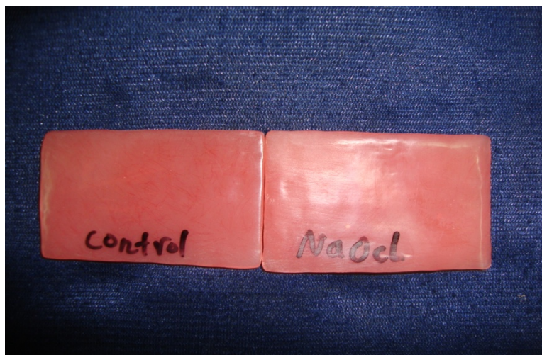
Figure 2: Photographs of specimens Immersed in distilled water and NaOCl
