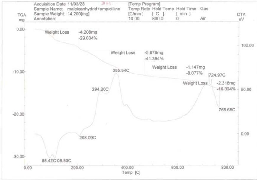
**Fig.(5) Thermal analysis( TG and TDA) of P2 drug polymer**
