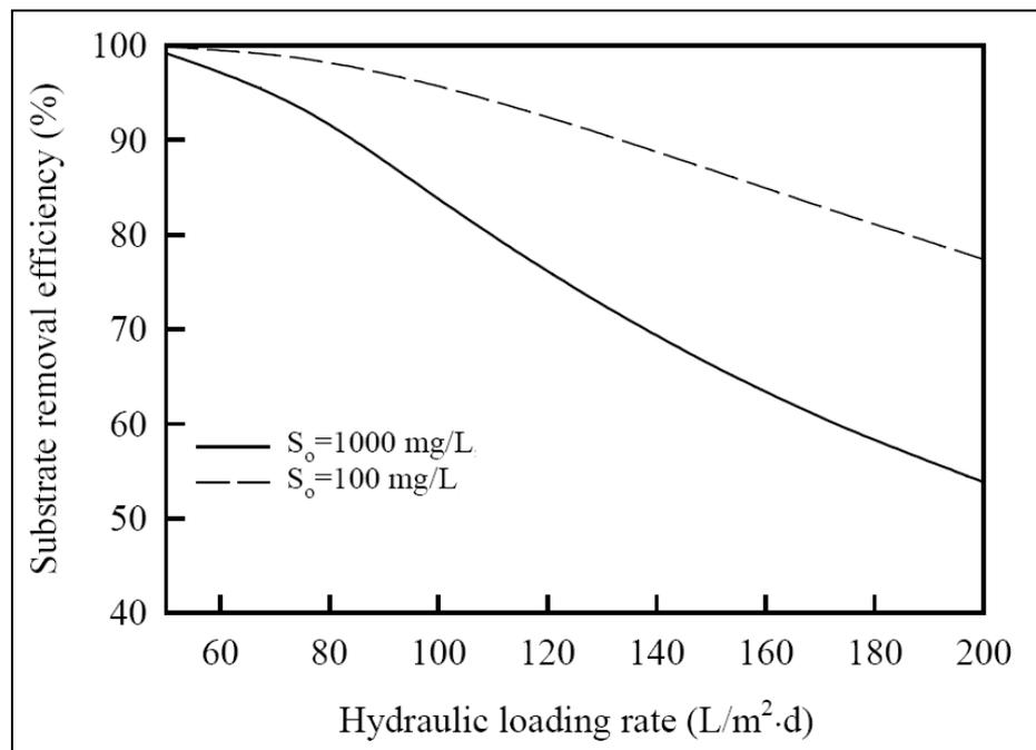
Figure 6: Effect of hydraulic loadings on the substrate removal efficiency at low and high inlet substrate concentrations.
