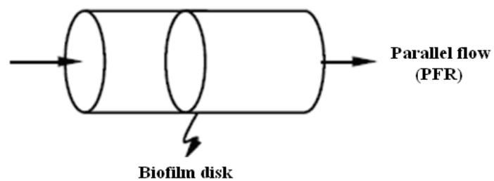
Figure 3. Representation of biofilm reactors (Plug Flow Reactor PFR)
