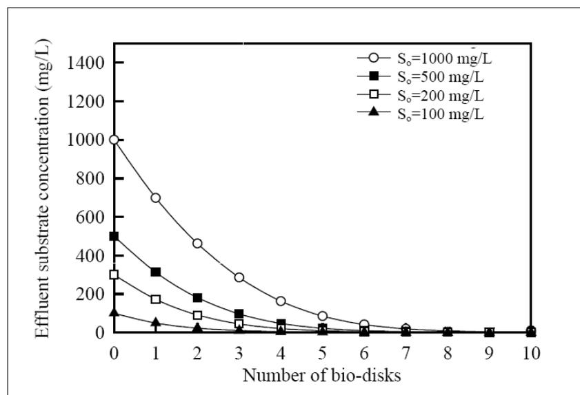
Figure 5: Effluent substrate concentration with respect to number of biofilm disks under different substrate inlet concentration
