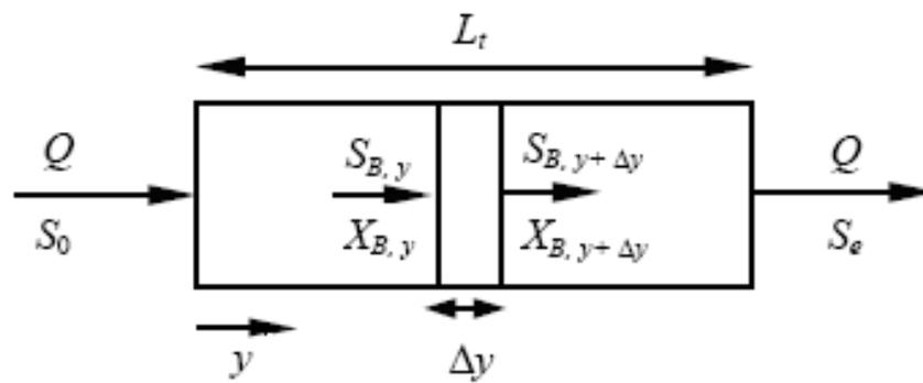
Figure 1. Schematic represent of a biofilm reactors.
