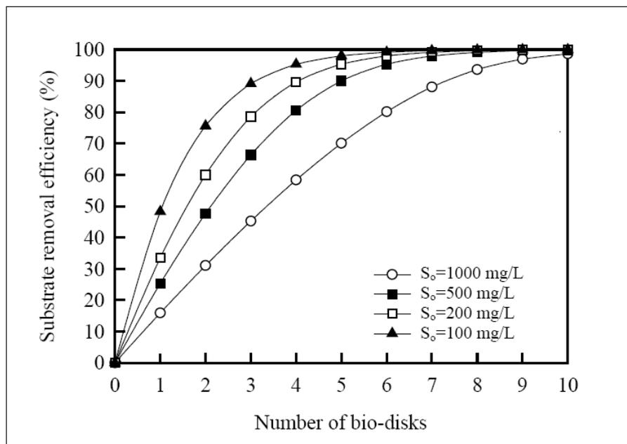
Figure 7: Effect of the number of bio-disks on substrate removal efficiency at different inlet
