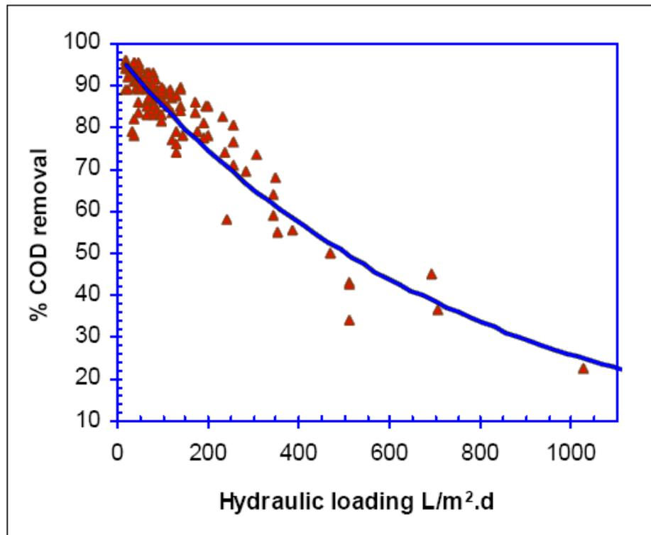
Figure 8: Effect of hydraulic loading on % COD removal.
