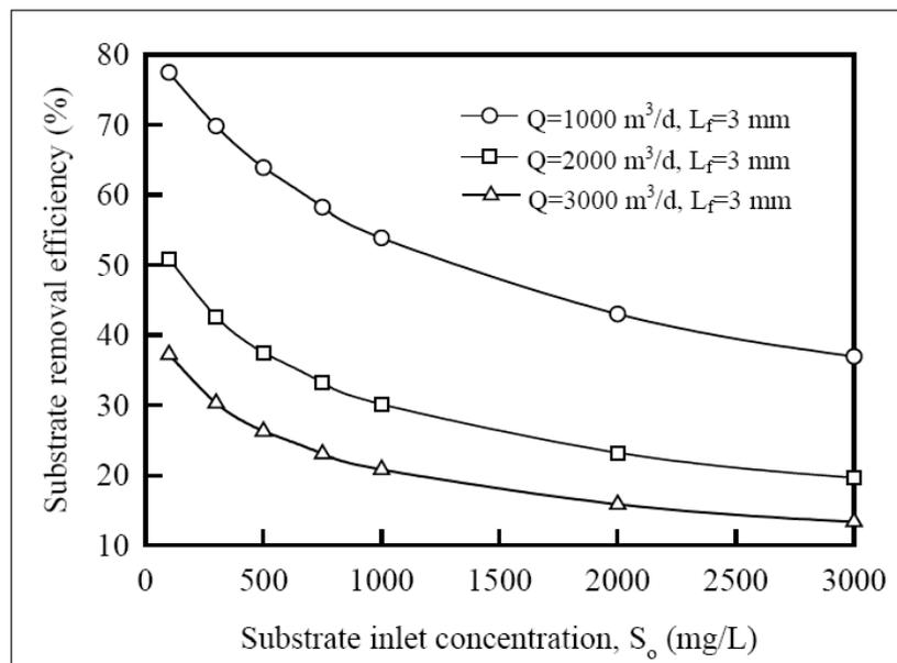
Figure 4: Substrate (BOD) removal efficiency with respect to inlet concentration under different flow rates and 3 mm biofilm active thicknesses.
