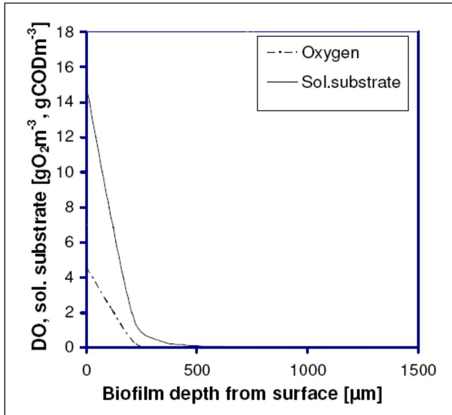
Figure 10: Concentration profiles of organic substrate, and dissolved oxygen inside the biofilm in RBC stages
