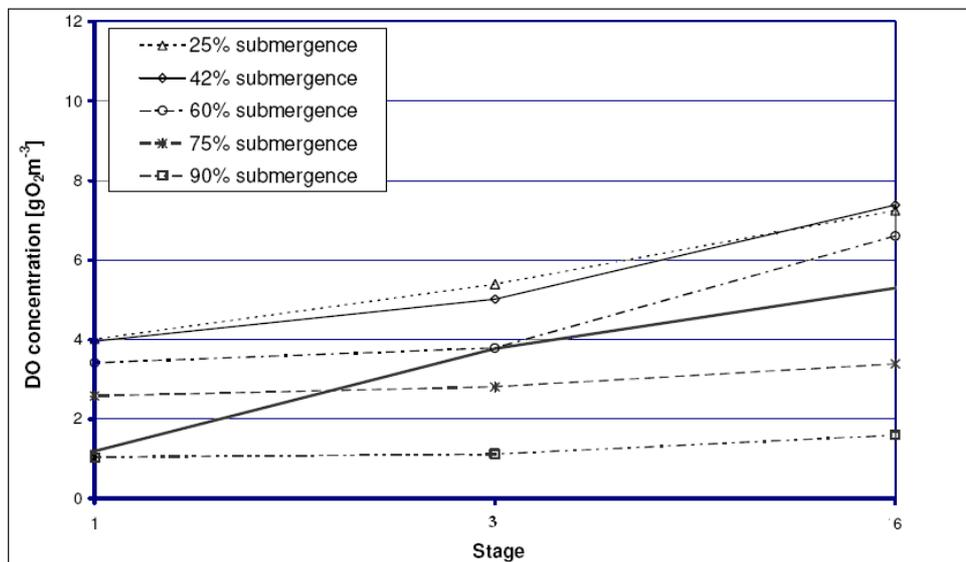
Figure 11: The DO concentration in bulk liquid under varying submergence ratio in RBC stages
