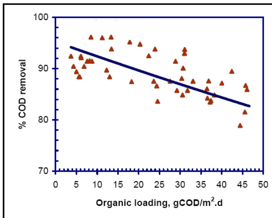
Figure 9: Effect of organic loading on the COD removal efficiency
