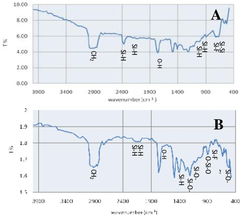
Figure (3): FTIR spectra showing the effect of ultrasonic treatment.
