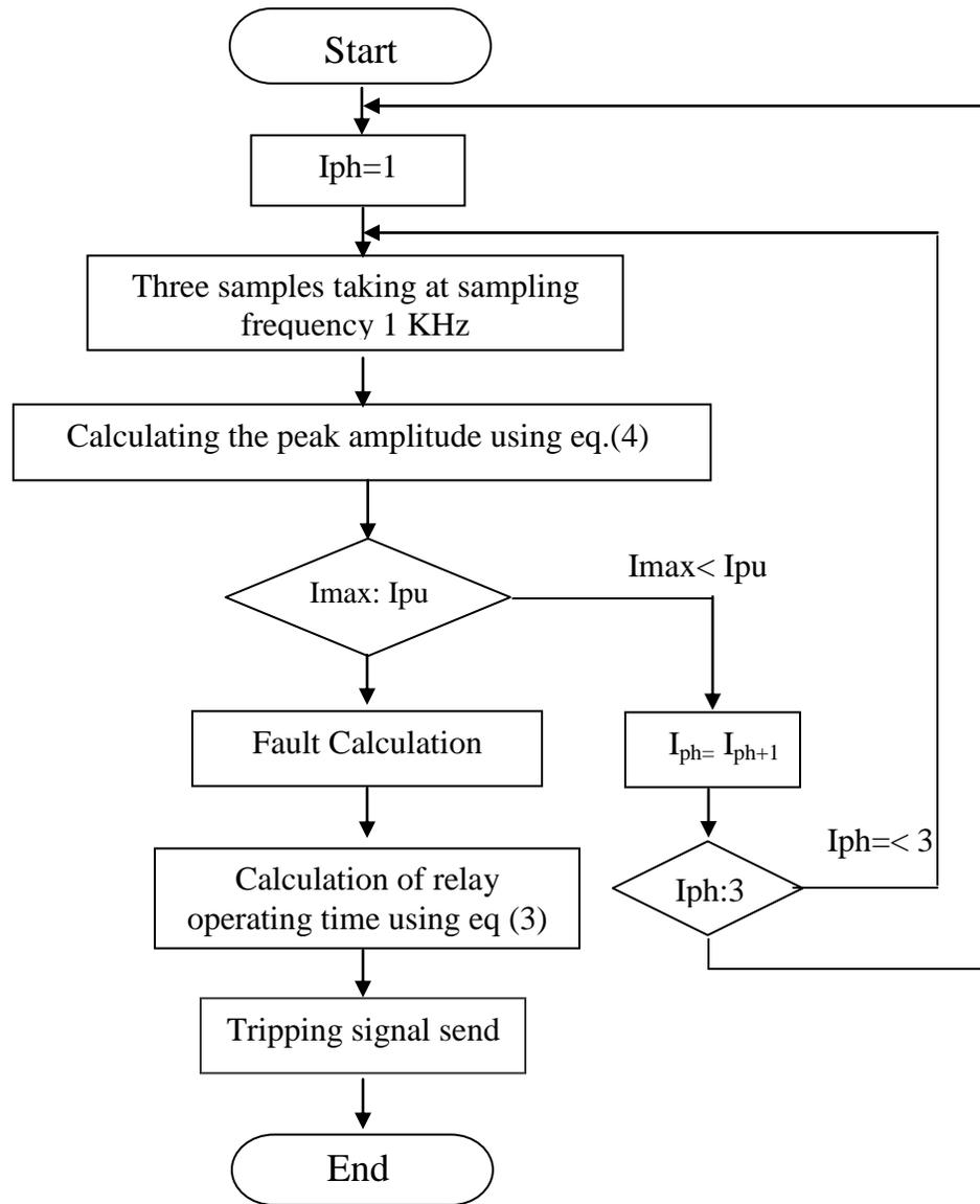
**Fig (4) Flow chart of overcurrent relay**
