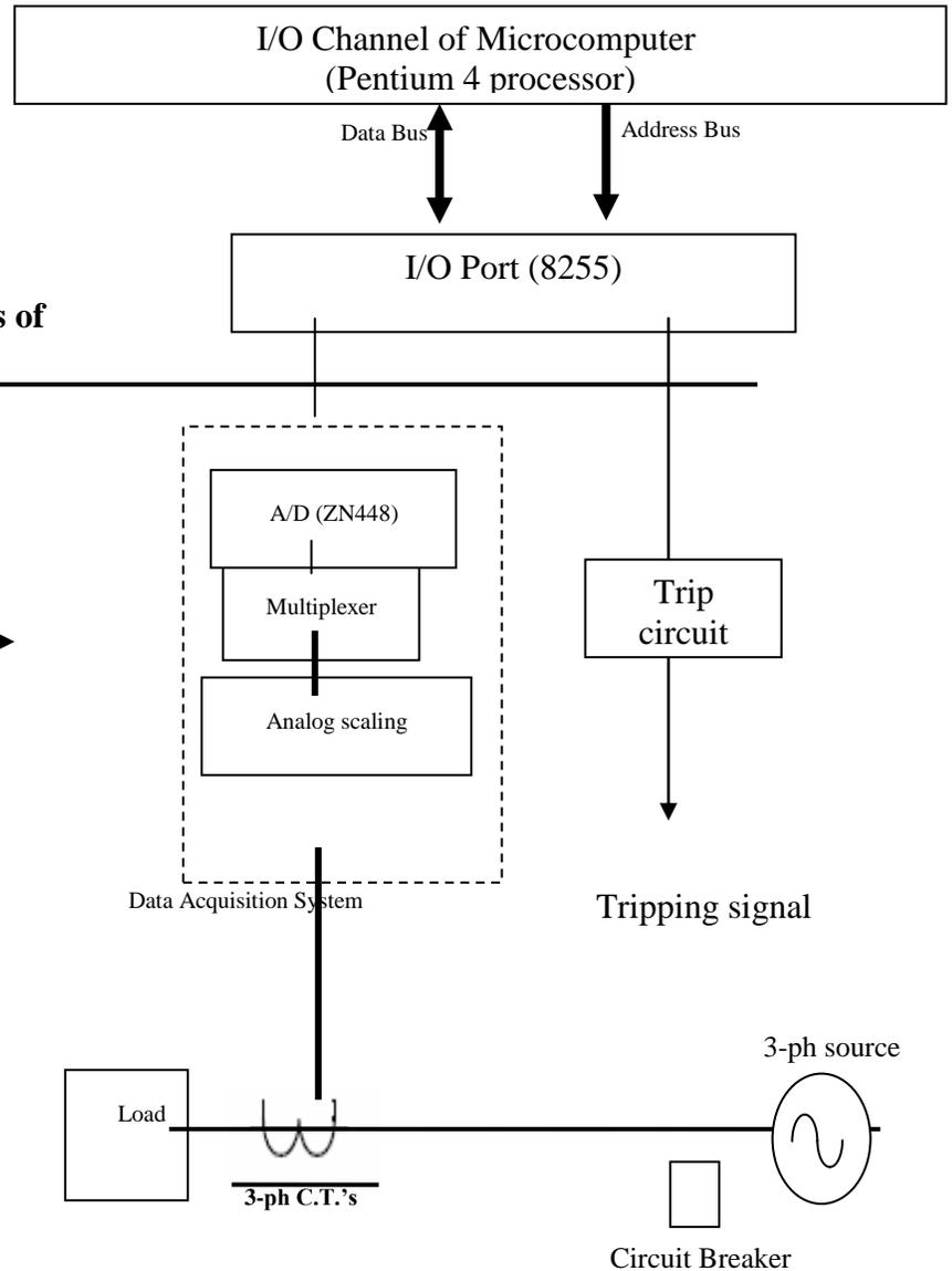
**Fig 3 Block diagram of the protection relay**
