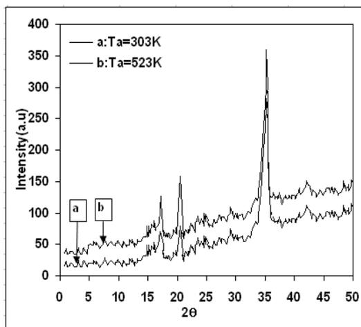
Fig. (1) XRD spectrum of the as-deposited  $In_2O_3$  thin films, and annealed at 523K
