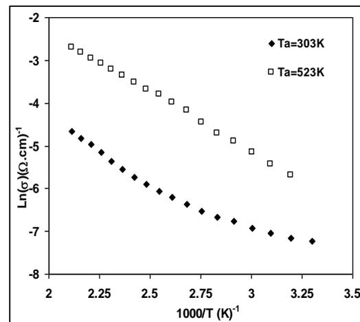
Fig. (2) Temperature dependence of D.C. conductivity  $\sigma$  of the as-deposited  $In_2O_3$  thin films, and annealed at 523K
