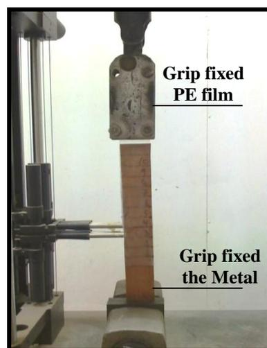
Fig (1): The specimen fixed between the grips
