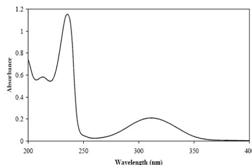
**Figure 1: UV- absorption spectrum of 5  $\mu$ g mL<sup>-1</sup> of phenoxazine in 12% ethanol.**
