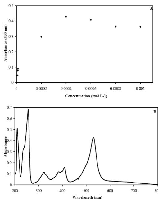
**Figure3: (A) Effect of the potassium metaperiodate concentration on the absorption at 530 nm of a phenoxazine solution of  $5 \mu\text{g mL}^{-1}$ . (B) UV-visible spectrum of the Oxidation product of  $5 \mu\text{g mL}^{-1}$  phenoxazine by using  $10^{-5} \text{ mol L}^{-1}$   $\text{KIO}_4$ .**
