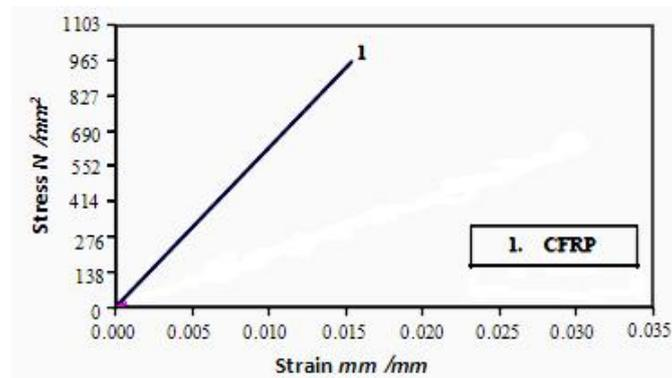
**Fig.(11):-** Stress-strain curves for the FRP composites in the direction of the fibers
