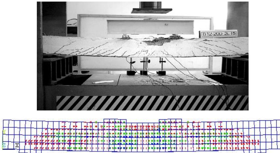
**Fig.(24):-** Cracks patterns in beam (12) and finite element model of beam( 12)
