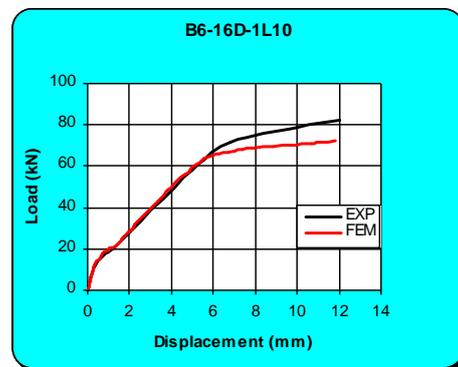
Fig.(13):- Load-deflection curve of beam (B6)
