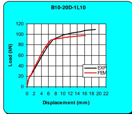
Fig.(17):- Load-deflection curve of beam (B10)
