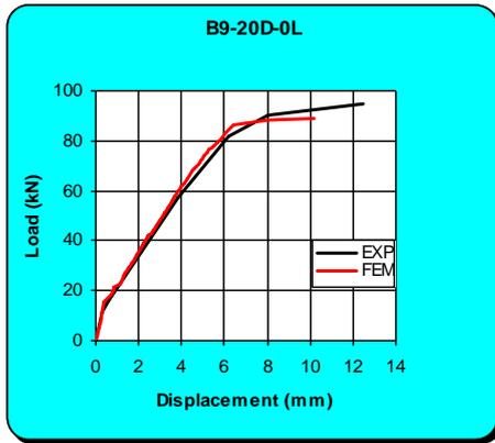
Fig.(16):- Load-deflection curve of beam (B9)
