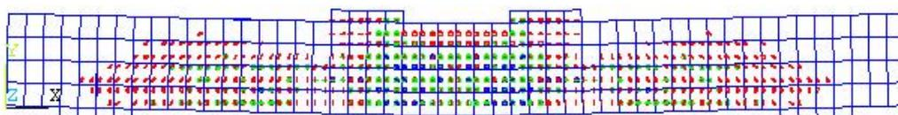
Fig.(23):- Cracks patterns in beam (10) and finite element model of beam( 10)
