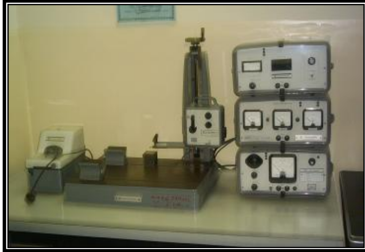
Figure (9) Roughness measurement apparatus
