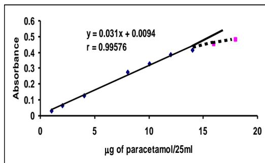
**Fig. 1: The calibration graph for paracetamol determination using the reaction between arsenazo III and cerium(III).**
