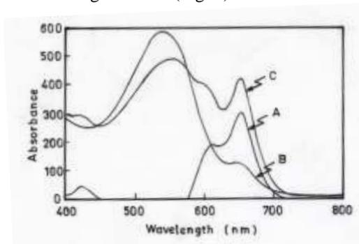
**Fig.2: Absorption spectra of  $10\mu\text{g}$  paracetamol / 25 ml treated according to the recommended procedure and measured against (A) blank, (B) distilled water and (C) blank measured against distilled water.**
