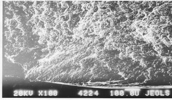
**Figure-6- Microphotograph of fatigue fracture surface**
