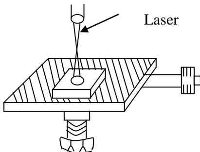
**Figure-2- Schematic illustration of a laser heat treatment configuration**
