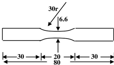
**Figure-1- Test specimen geometry and dimensions (all in mm).**
