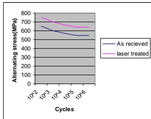
**Figure –5- Relation between applied cyclic stress and number of cycles.**
