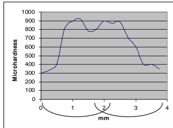
**Figure-3- Hardness distribution in the overlapped double pass specimen.**
