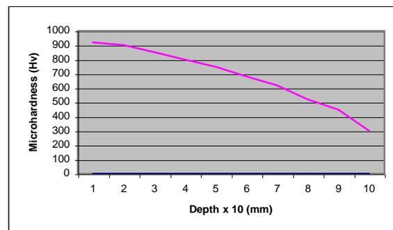
**Figure-4- Depth of hardening.**
