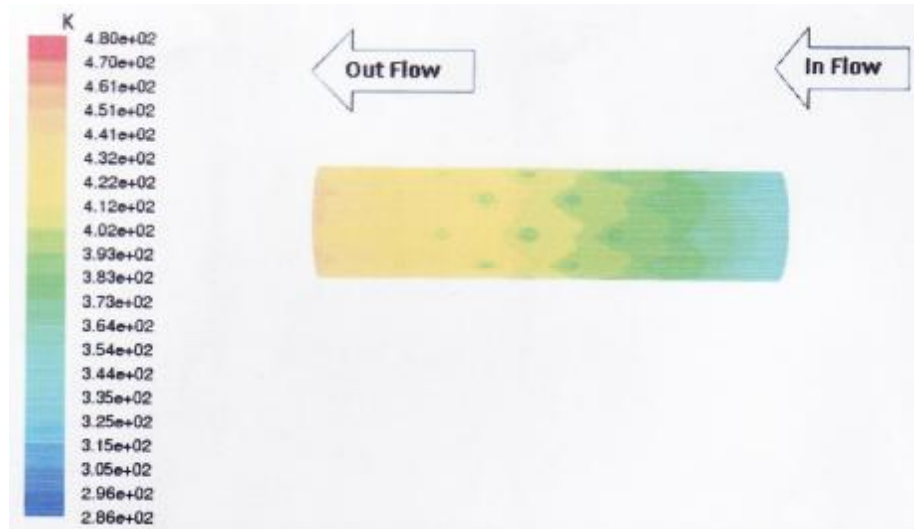
Figure (18) Temperature contour on outer Cylinder heated surface ( Re=6774 )
