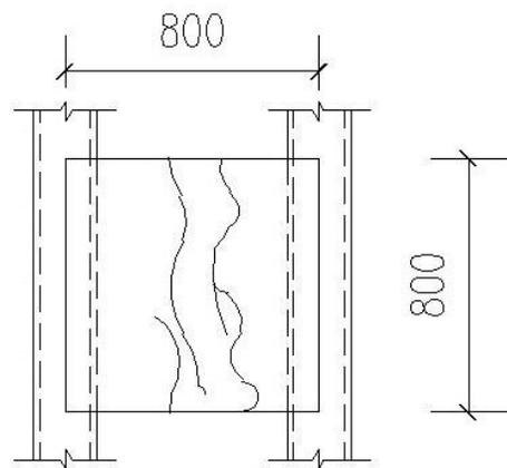
**Fig.(7):** The crack pattern (S<sub>4</sub>).
