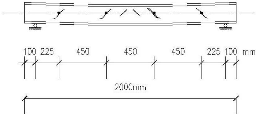
**Fig. (4):**Bolt position and the cracks pattern.
