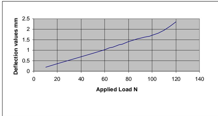
**Fig. (3):**Measured deflection values versus applied loads .
