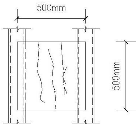
**Fig.(5):**The crack pattern ( $S_2$ ).
