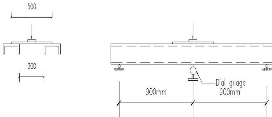
**Fig. (2):**Tow edges simply supported beams.
