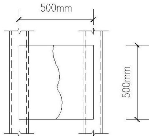
**Fig.(6):** The crack pattern (S<sub>3</sub>).
