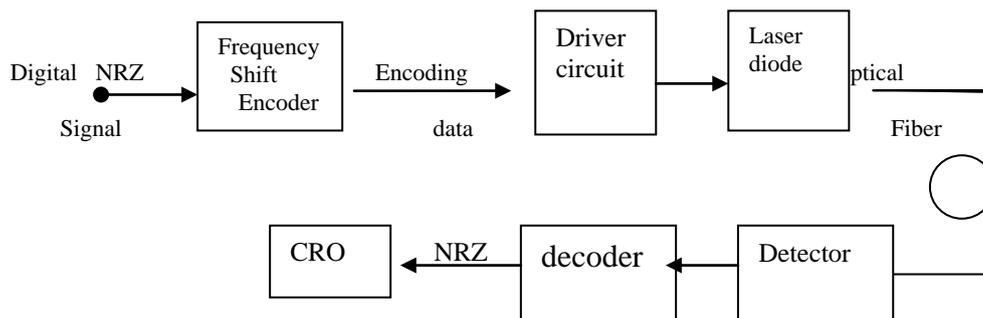
Fig.(2):General Block Diagram of Frequency Shift Coding System
