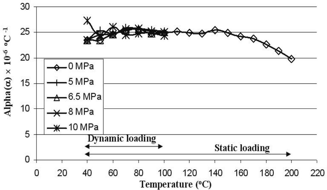
Fig.(4) : Coefficient of thermal expansion of PbSb alloy vs. temperature for different loading stresses.
