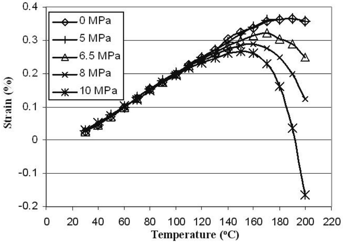
Fig.(3) : Strain behavior vs. temperature for PbSb alloy at different applied stresses.
