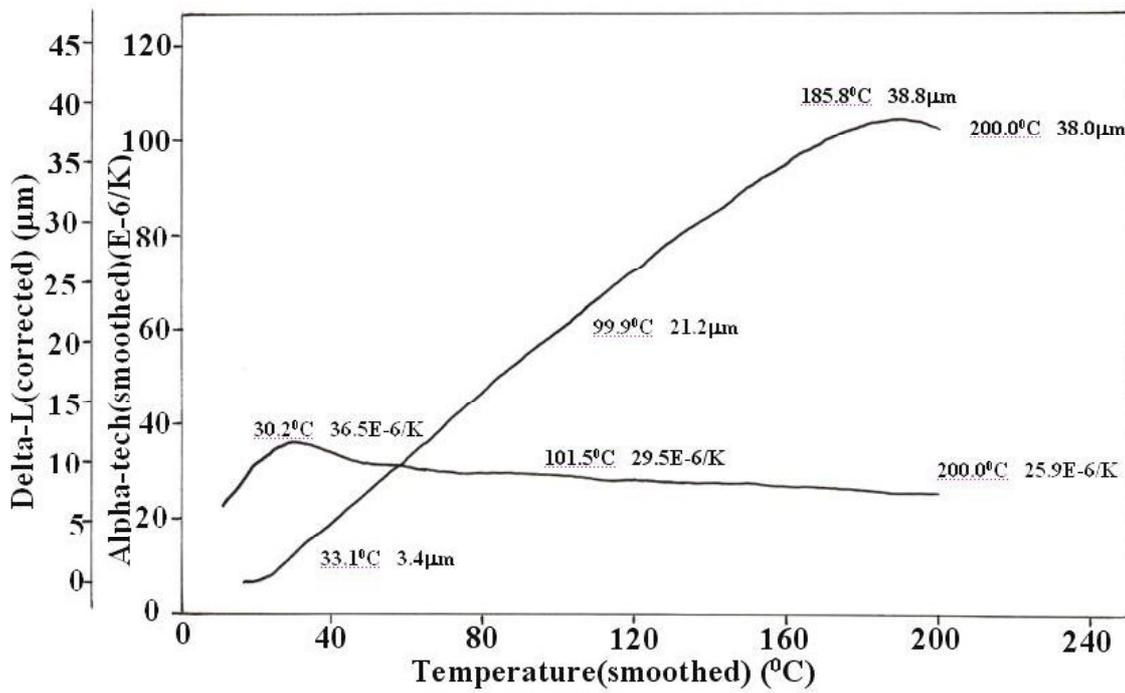
*Fig.(2) : Typical TMA chart for PbSb alloy showing multi-axes ( $\Delta L$  and  $\alpha$ ) behavior as a function of temperature.*
