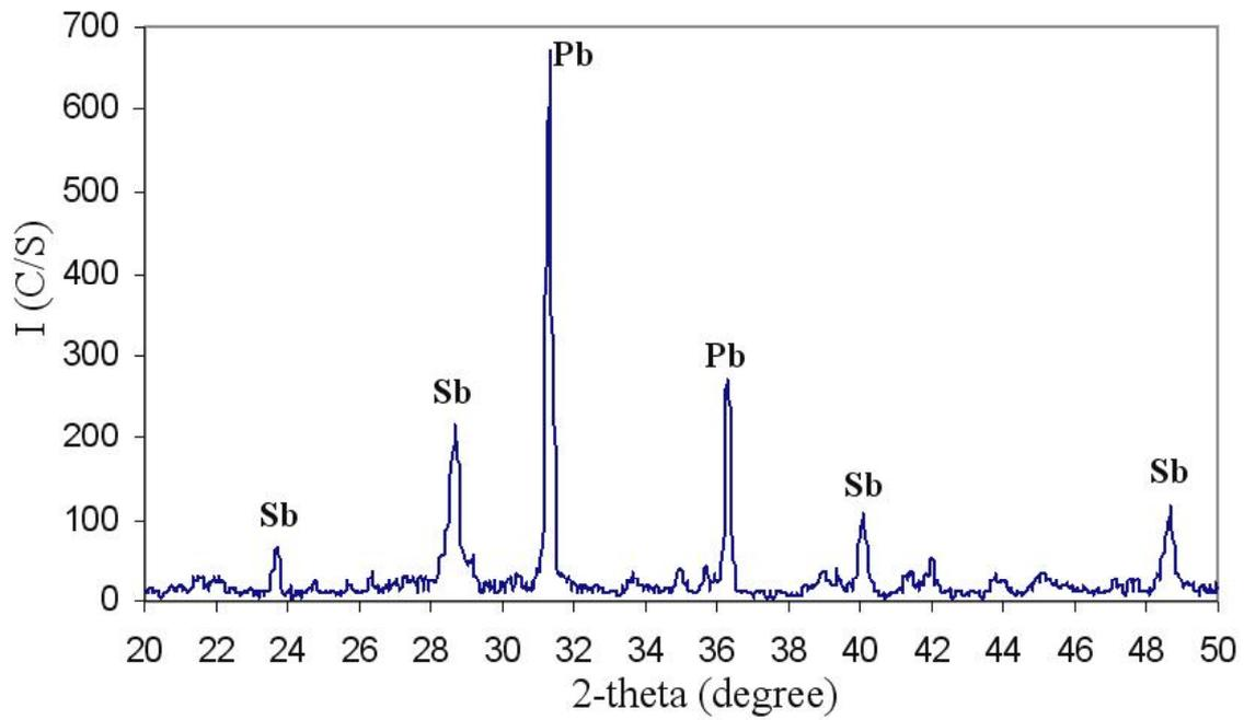
*Fig.(1) : XRD Spectrum of Eutectic PbSb alloy.*
