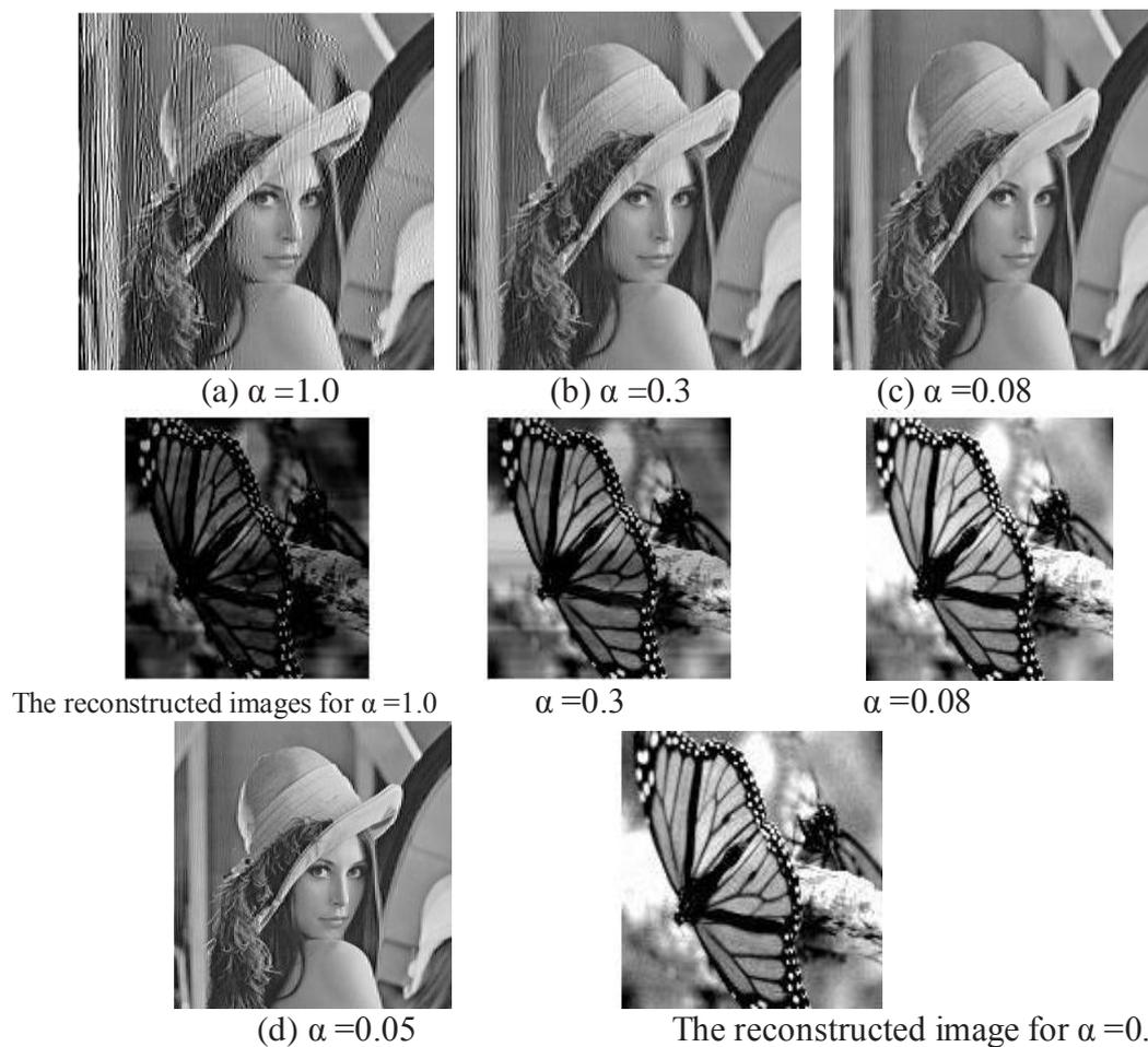
**Fig. (7) Embedded images using the butterfly image as signature at varying scale factors and the reconstructed butterfly image.**
