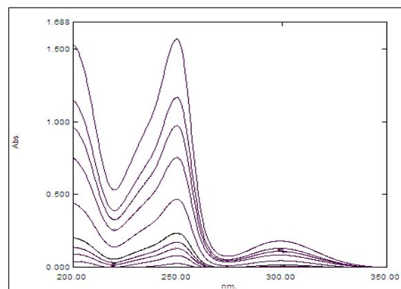
**Fig.(7) Spectra for Promethazine hydrochloride solutions at different concentration ranged from 2 to 62 mg/L.**
