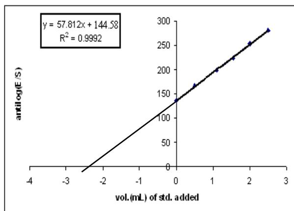
**Fig.(5) Plot of antilog (E/S) versus the volume of promethazine using metode using promethazine hydrochloride selective electrode using DBPH plasticizer.**
