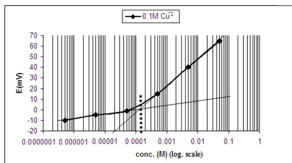
**Fig.(4) Calibration curve of fixed interfering method using promethazine hydrochloride selective electrode using DBPH plasticizer.**
