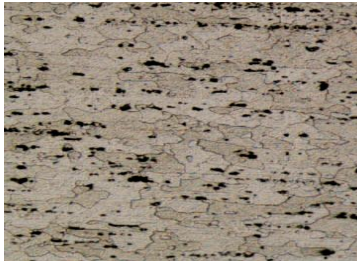
Figure (5) Microstructure of Fe-4% Cu alloys after air -cooled. (Massive Ferrite with precipitates of Cu and some Particles of Fe 2 O 3 or Cu 2 O). (X200)
