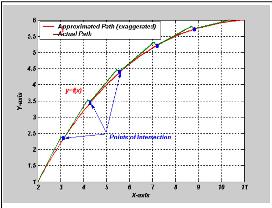
Figure (7) Exaggerated tool path of BLCA technique (Example I)
