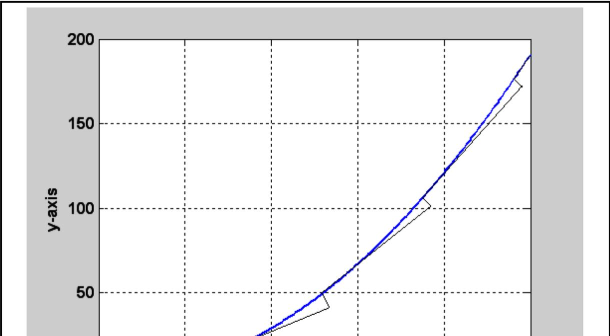
From the previous Figure (7) it is obviously noted that tool path generated from BLCA approach suffers from an important drawback that is over-cut metal left by the cutter during the translation from the end path to the next one. This over cut metal depends on the cutter diameter and the angle of lab as shown in Figure (11).
