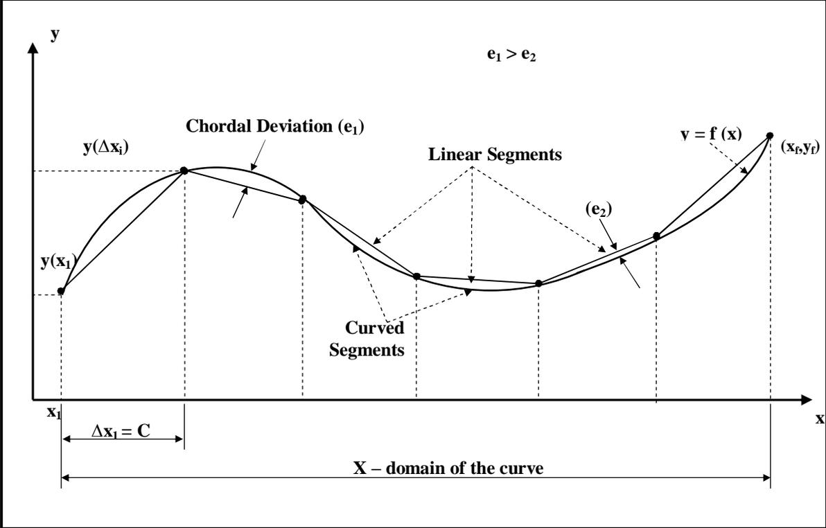
**Figure (3)** Schematic representation of ILCA procedure, shows a fluctuation of chordal deviation from high to low along the X-domain of the curve.
