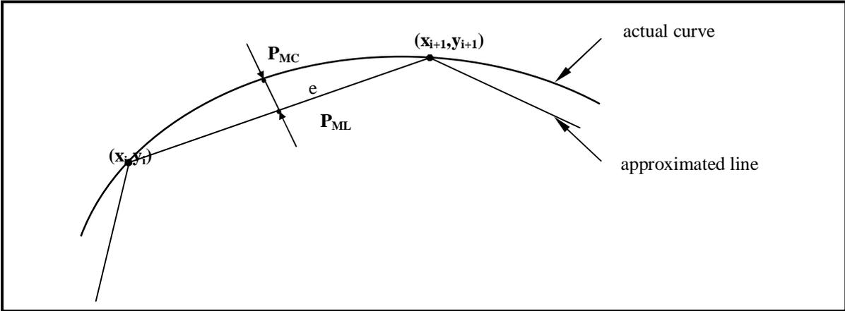
**Figure (4)** (Exaggerated) chordal deviation between the actual curve and approximated line
