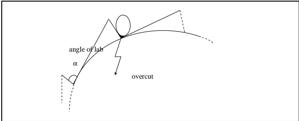
**Figure (11)** over-cut area as the drawback of BLCA approaches
