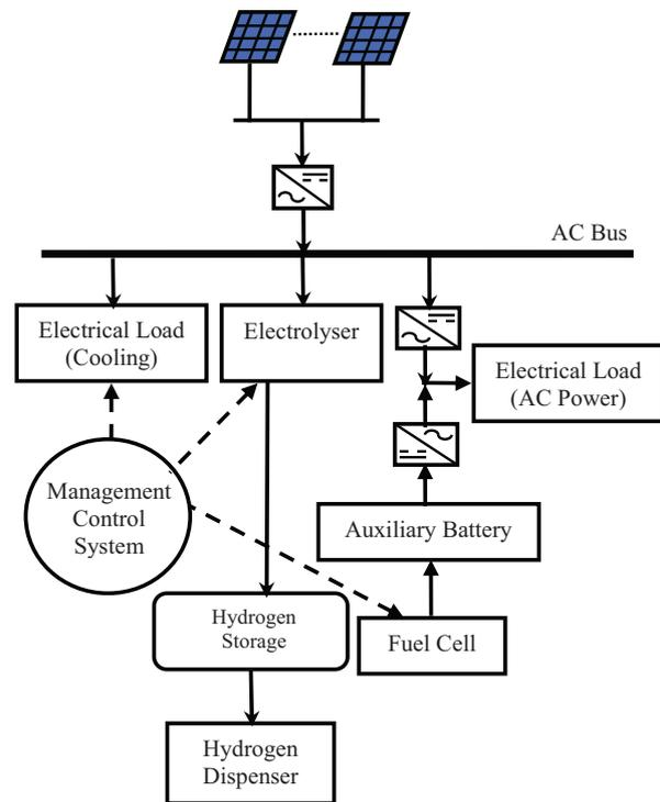
Fig. 6 Basic components of Middle East version of Unst integrated renewable energy system
