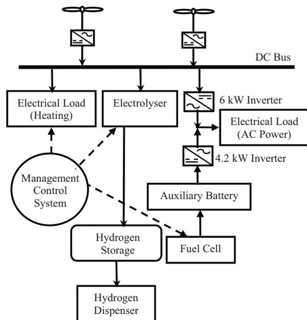
Fig. 2 Basic components of Unst integrated renewable energy system
