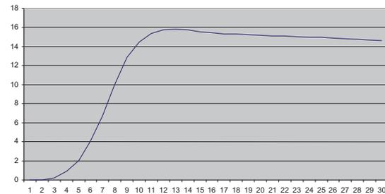
Fig. 3 Power curve for 15kW Proven wind turbine
