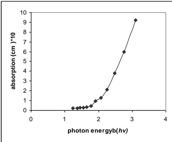
Fig. (3) : The absorption coefficient versus photon energy of films.
