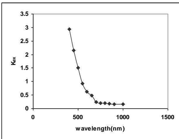
Fig. (5) : The extinction coefficient ( $K_{ex}$ ) versus wavelength.
