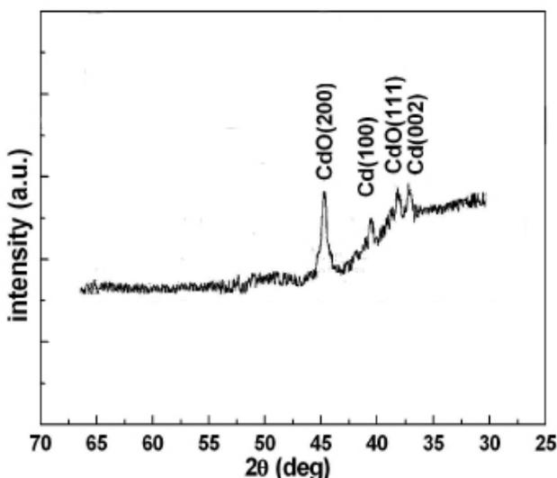
Fig. (1): XRD patterns (CuK $\alpha$  radiation) of CdO thin films deposited at substrate temperature of 300 K.
