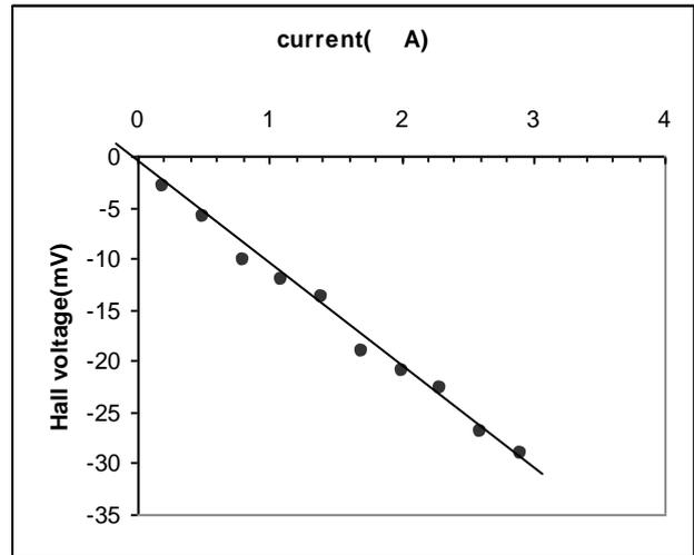
Fig. (6) : Hall voltage vs current pass through CdO thin film.
