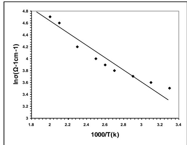
Fig. (7) : Reciprocal temperature dependence of electrical conductivity for CdO thin films.
