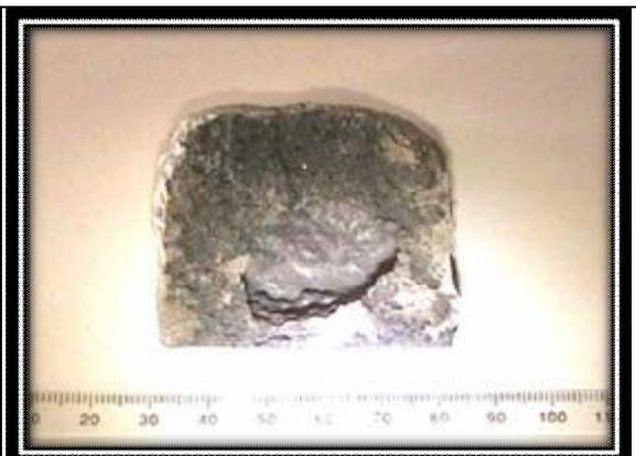
Figure(12): ample foamed for(15min). The mechanism of foam formation is a function of foaming time <sup>[4]</sup>, but the metallic foams are unstable systems because their large surface area causes energy to be far from a minimum value <sup>[13]</sup>
