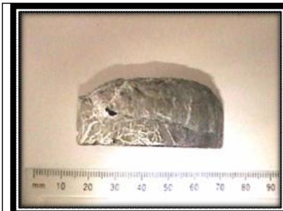
Figure(11) Sample foamed for(5min)
