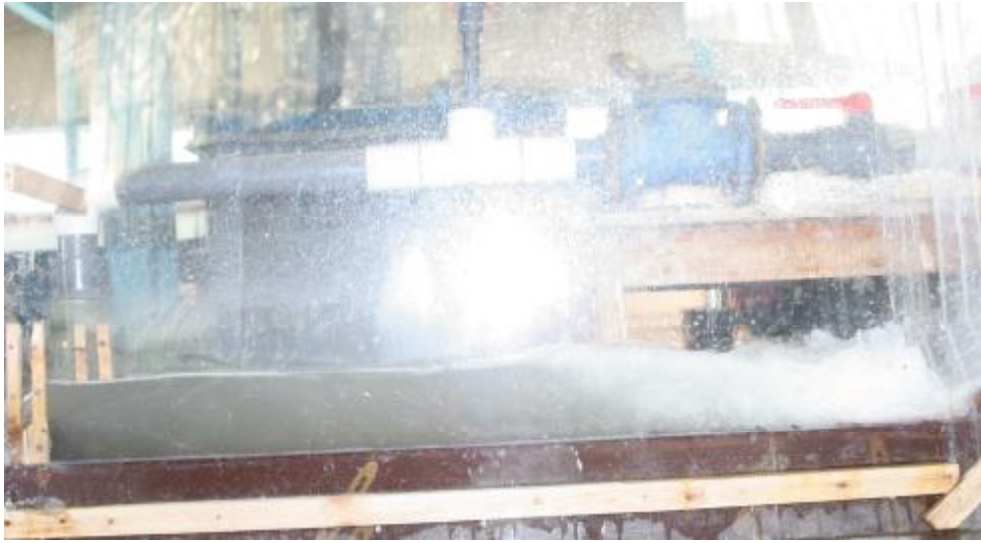
Figure (5) The hydraulic jump forced at a stilling basin.
