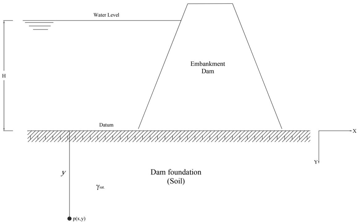
Figure(2): Effective stresses at a point below embankment dam
