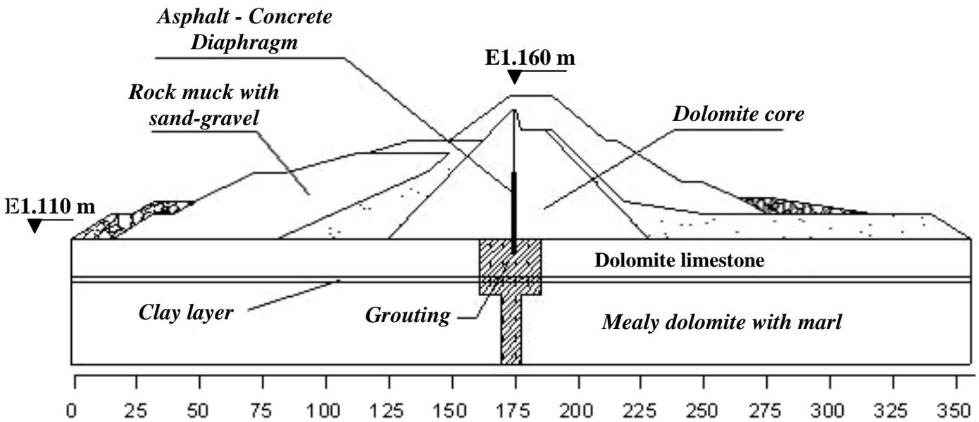
Figure(5): Typical cross section of Haditha Dam with ground profile
