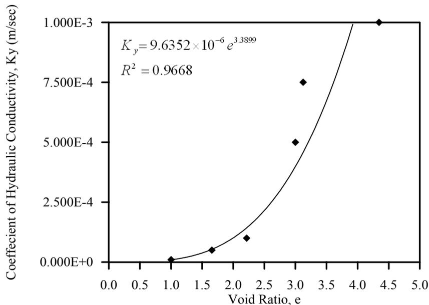
Figure(3): Vertical permeability vs. void ratio relationship for sandy soil
