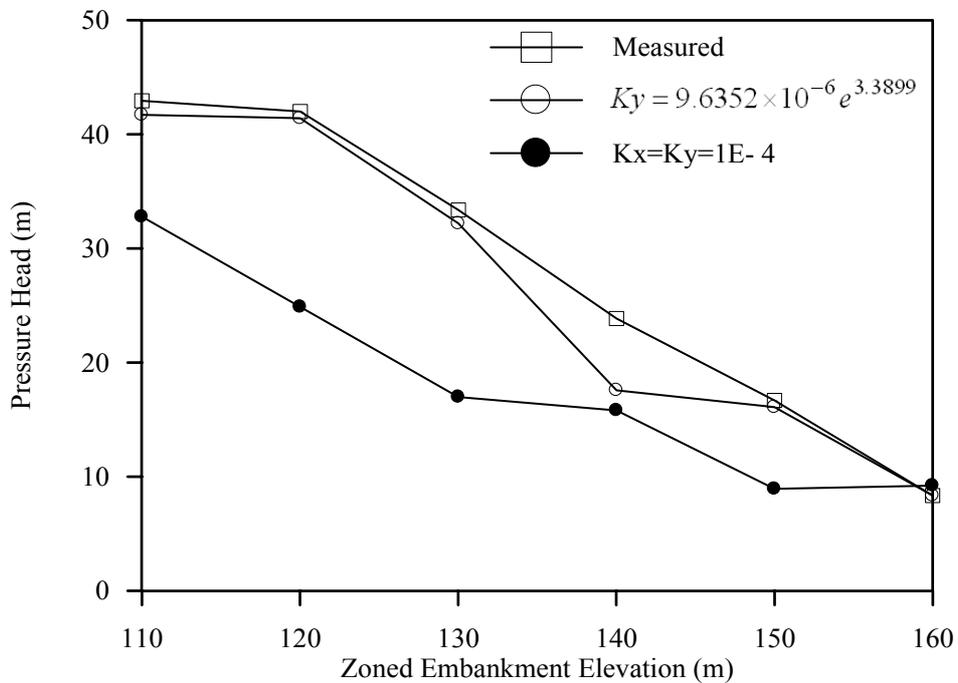
Figure(7): Influence of variation of permeability on pressure heads distribution in section (1-1) for various dam levels in the U/S face.
