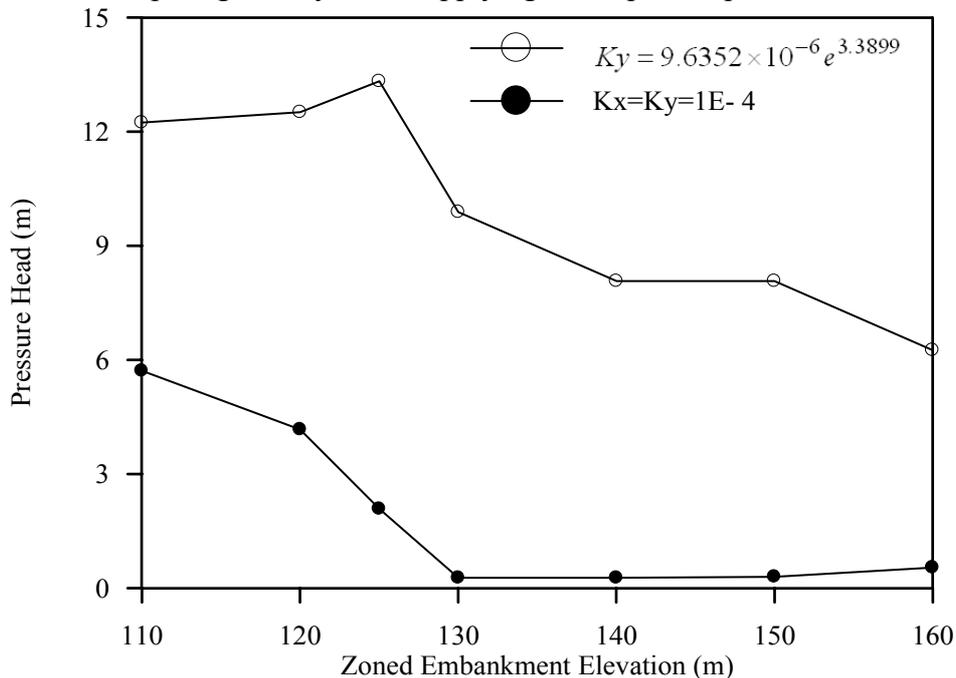
Figure(9): Influence of variation of permeability on pressure heads distribution in section (3 - 3) for various dam levels in the D/S face.
