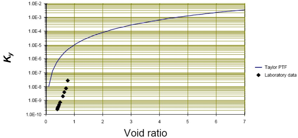
Figure(1) : Void ratio versus coefficient of permeability for sandy clayey soil(Leroueil *et al.*,1992)
