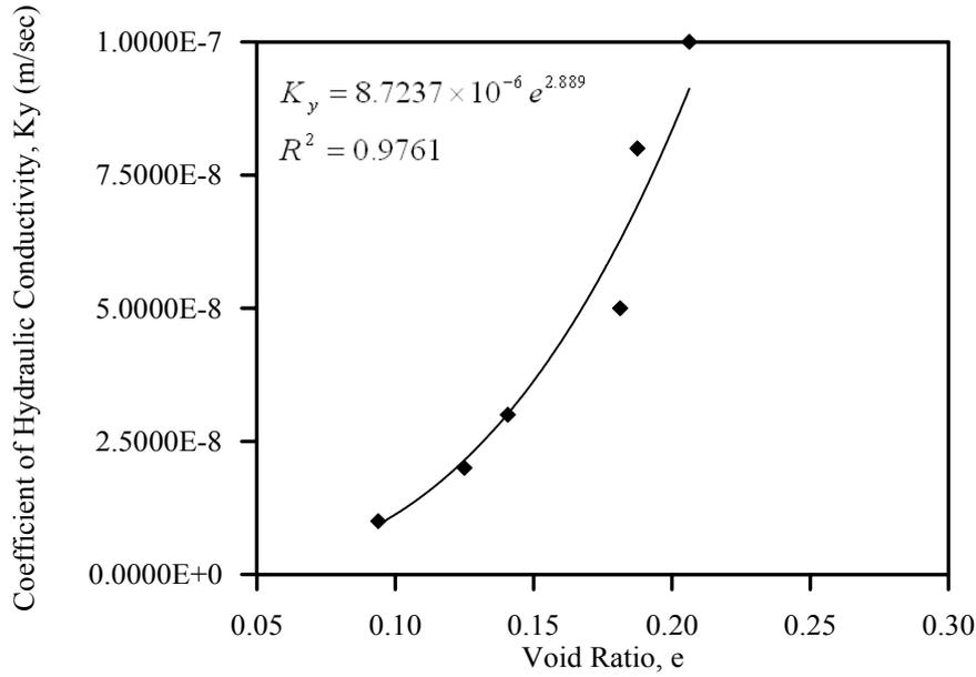
Figure(4): Vertical permeability vs. void ratio relationship for clayey soil
