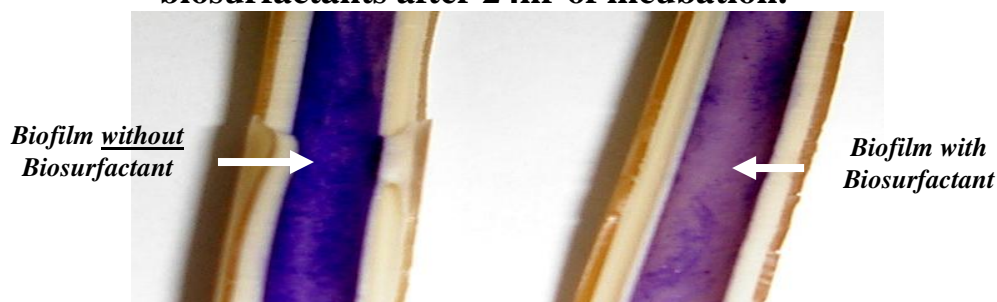
Fig. 4: Stained Enterococcus faecalis biofilm on Foley catheter with and without biosurfactants after 24hr of incubation
