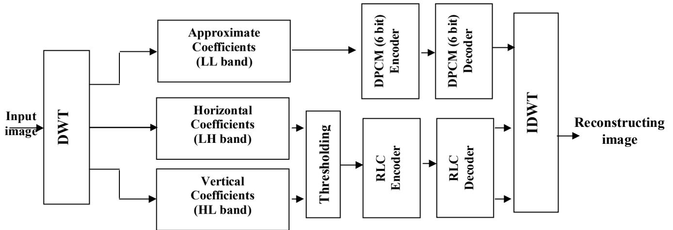
**Fig.(5) Image compression and decompression system using DWT and RLC**
