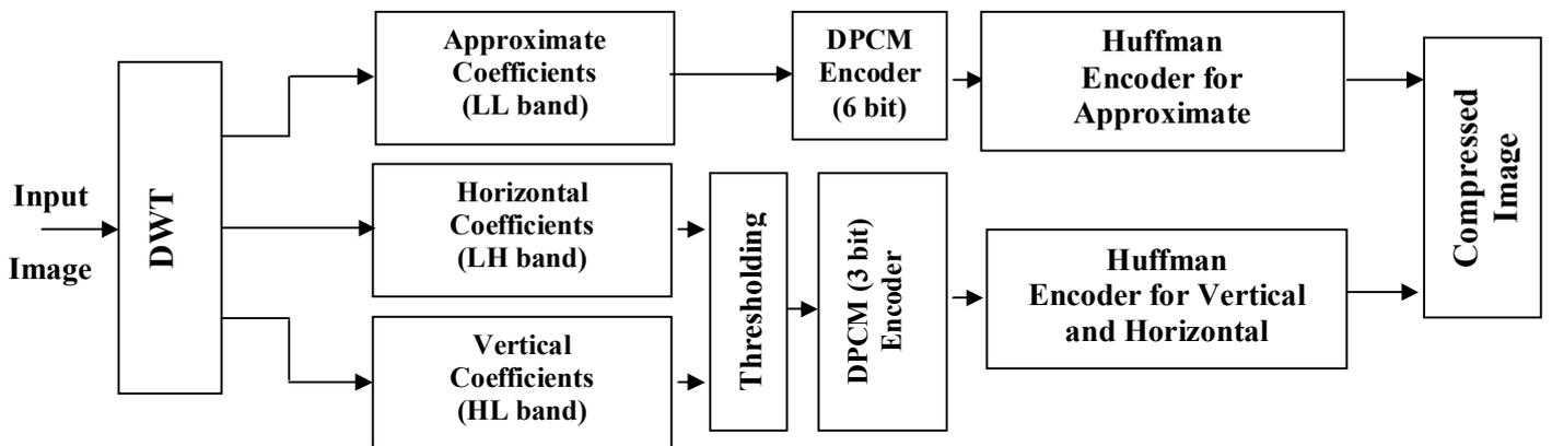
**Fig.(6a) Image compression technique using DWT and Huffman code**
