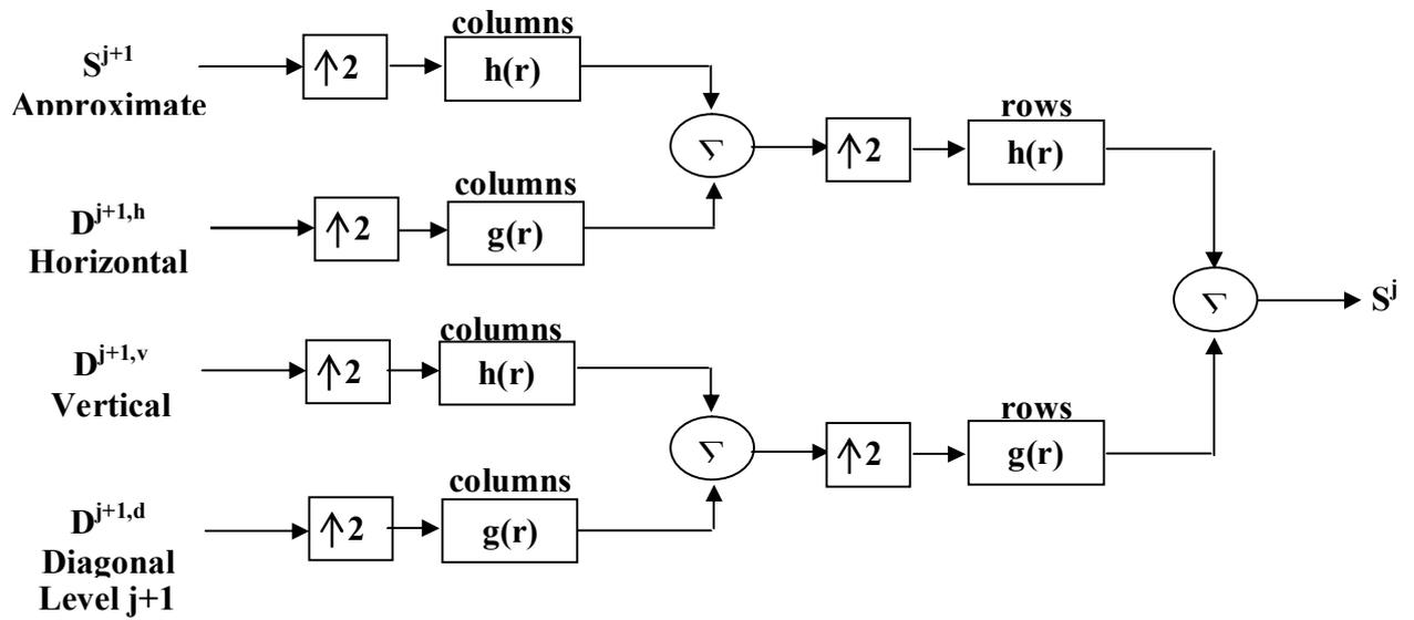
Fig.(2) Inverse discrete wavelet transform (synthesis)
