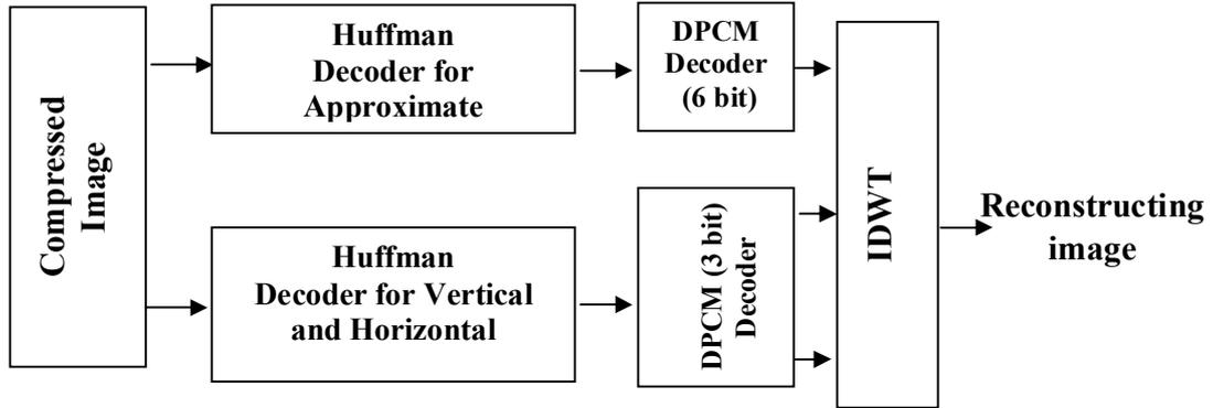
**Fig. (6b) Image decompression technique**
