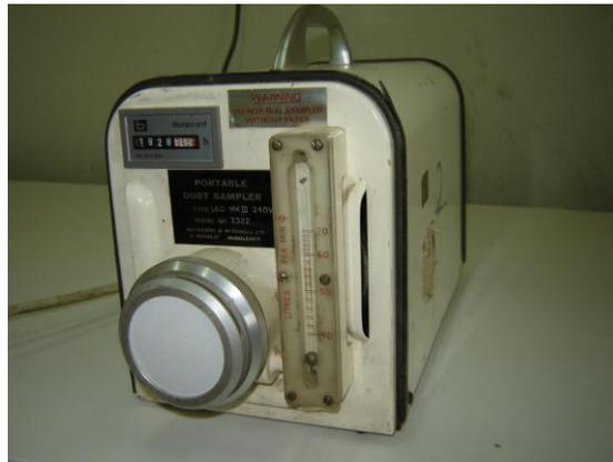
Fig.(1): Portable dust sampler (Sniffer, L-30)
