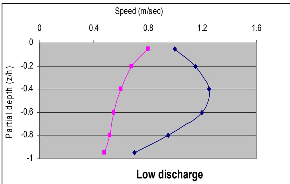
Fig. 5: Current speed distribution during the high and low discharge at Al-Fao station (flood  $\blacklozenge$ , ebb  $\blacksquare$ ).
