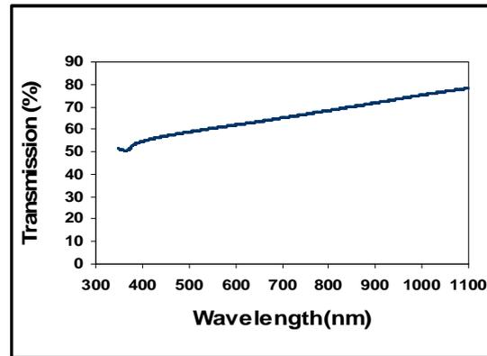
Fig. ( 3 ): The transmission spectra of ZnO thin films
