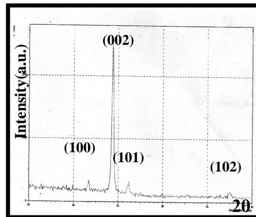
Fig. (2): X-ray diffraction pattern (XRD) pattern of ZnO thin film before annealing
