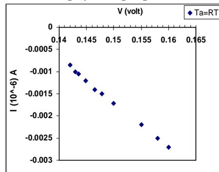
Fig. ( 11 ): The plot of Hall voltage versus the current for ZnO Thin Films
