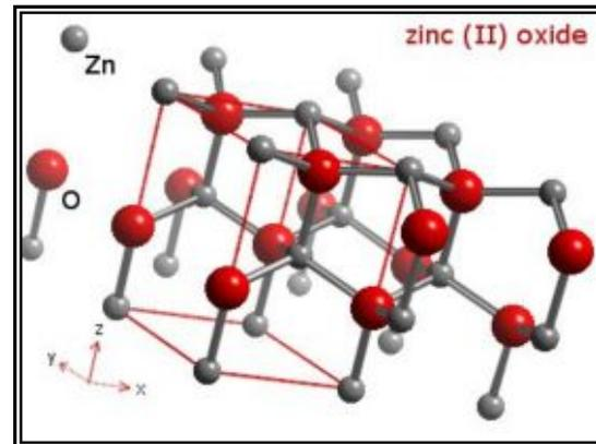
Fig. (1): The crystal structure of ZnO
