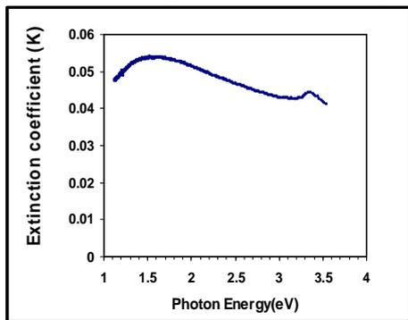
Fig. ( 9 ): The extinction coefficient of ZnO thin films
