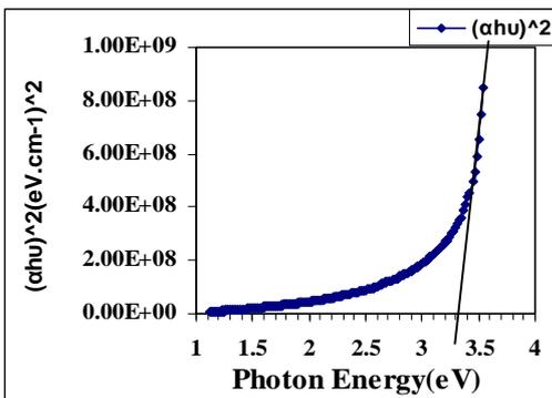
**Fig. (5): The direct allowed transition energy gap of ZnO thin films**
