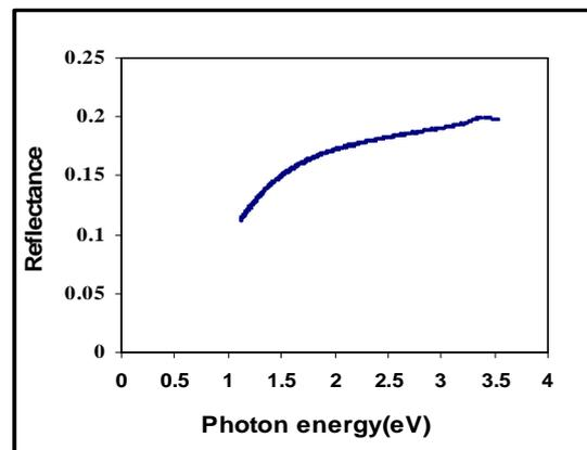
Fig. ( 4 ): The reflectance spectrum of ZnO thin films as a function of the photon energy
