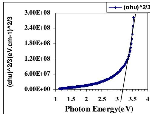
**Fig. (7): The energy gap for direct forbidden transition of ZnO thin films**
