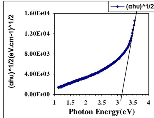
**Fig. (6): The optical energy gap of ZnO thin films for the indirect allowed transition**
