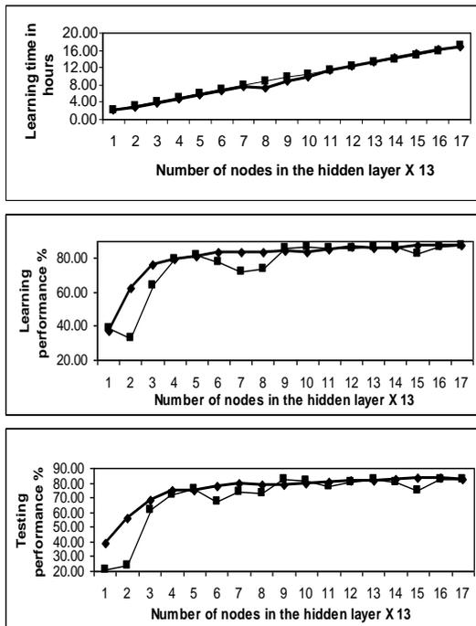
Fig.-3: The comparison of one-against-all versus the ordinary architecture. The upper chart shows the training time for one-against-all is slightly better than the ordinary one. The training and testing performance for one-against-all are little better than the ordinary one. Dark lines represent the one-against-all while the light lines represent the ordinary scheme.
