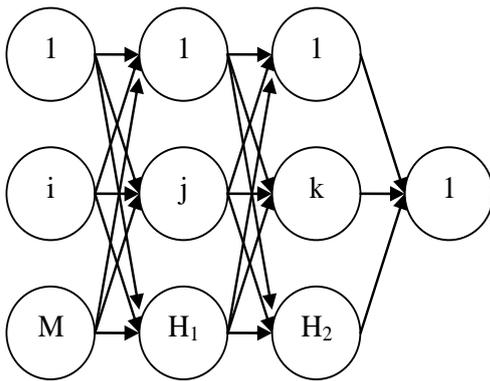
Fig.-2: The architecture of the one-against-all network. Thirteen of this ANNs have been trained. One for each class. During classification, we present the input for each one. The class will be adapted from the one with the highest score
