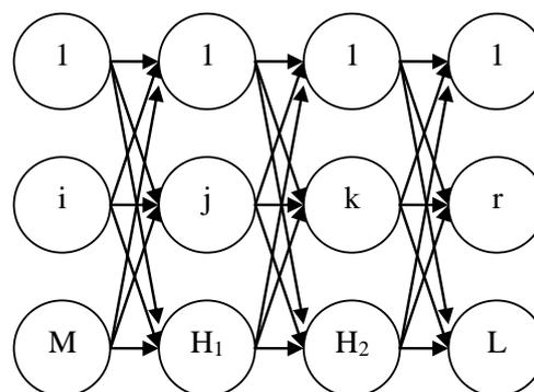
Fig.-1: The architecture of an ordinary MLP with two hidden layers. Number of nodes in the input layer, the first hidden layer, the second hidden layer, and the output layer are M, H<sub>1</sub>, H<sub>2</sub>, and L, respectively
