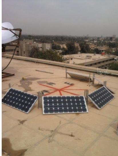
Fig ( 5 ) shows the five solar panels installation in five direction
