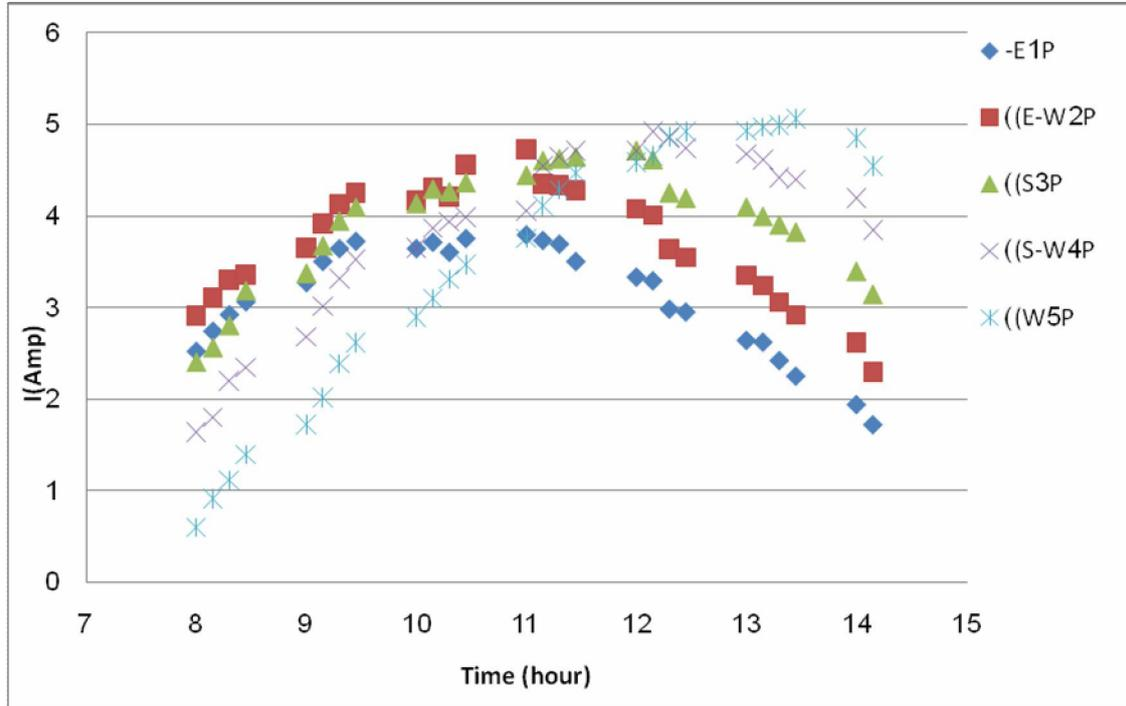
Fig (7) shows the output solar panels (current) with the time
