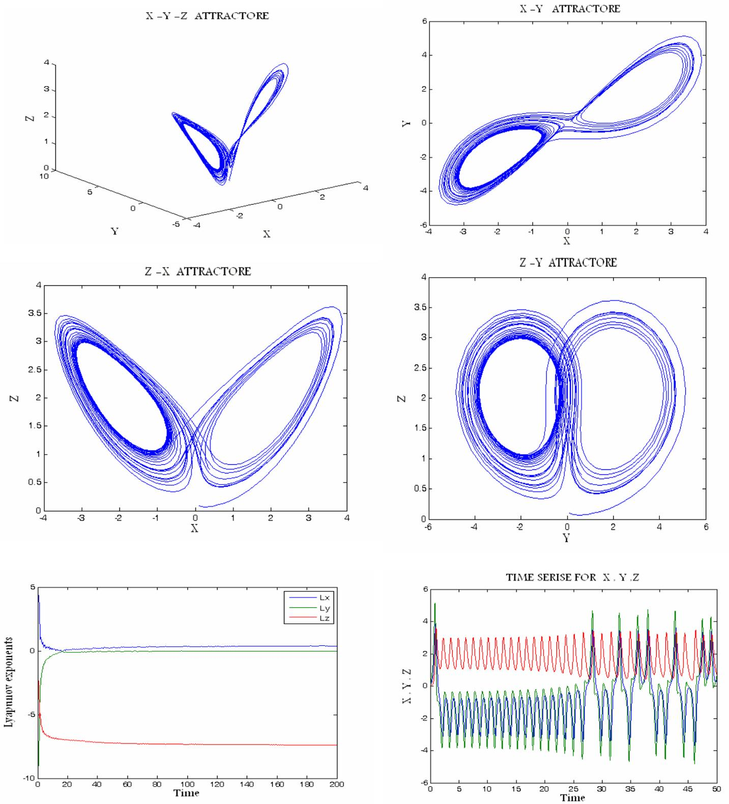
Fig : (2a) : Three dimensional (a) and two dimensional (b,c,d)attractors , Lyapunov exponents (e) and time series (f) for  $a=5, b=2.1, c=2$
