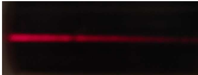
Figure (6) Experimental demonstration of self-focusing propagation in the cell of natural red dye molecule.
