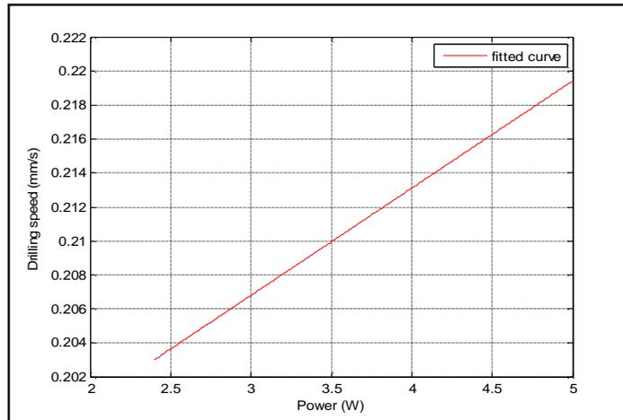
Figure (6) The relation between laser power and drilling speed for wood using CO<sub>2</sub> laser
