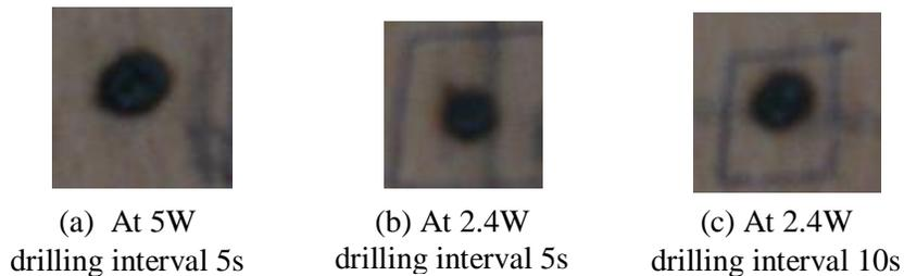
**Figure (5) Wood drilled by CO<sub>2</sub> laser**
