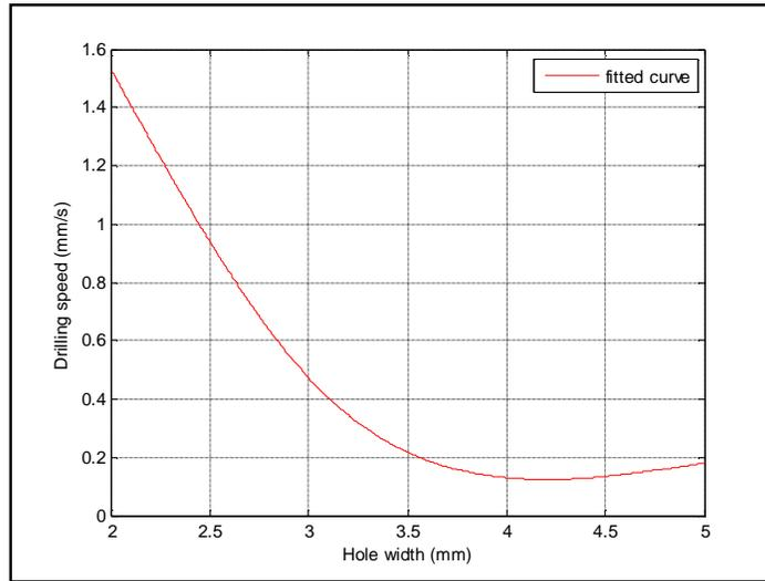
**Figure (8)** The relation between hole width and drilling speed for wood using CO<sub>2</sub> laser
