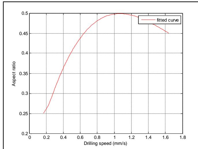
**Figure (9)** The relation between drilling speed and aspect ratio for wood using CO<sub>2</sub> laser
