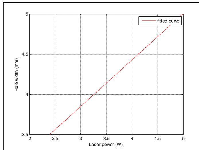
Figure (7) The relation between laser power and hole width for wood using CO<sub>2</sub> laser
