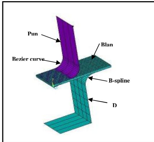
Figure (6) The finite element model of U-bending
