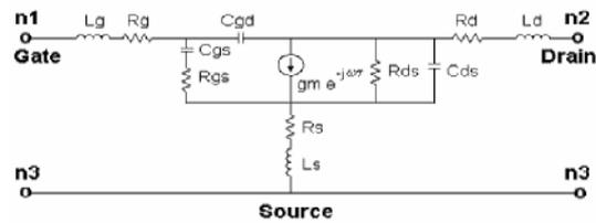
Fig. (10) A simplified equivalent T-model for the InZnO TFT
