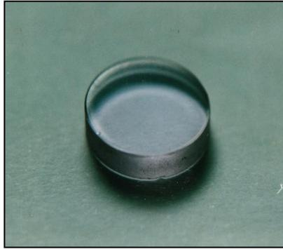
**Figure (1-5): The Laser Active Medium**
