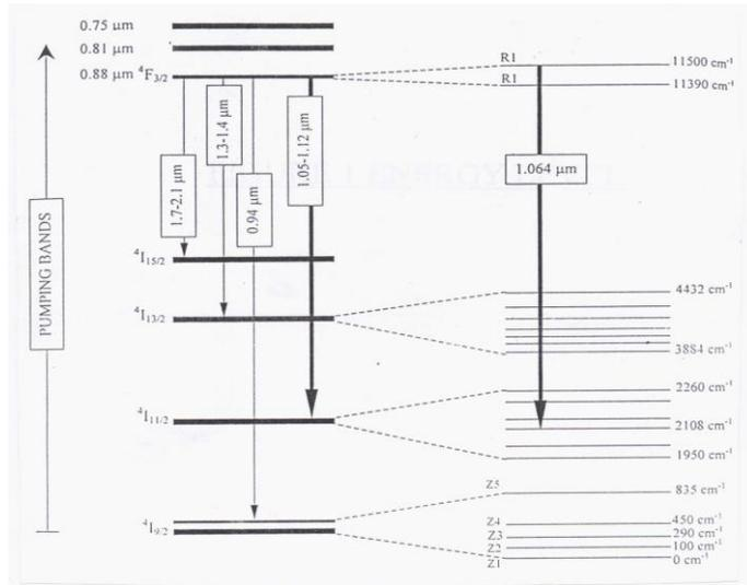
**Figure 1-1: Schematic Diagram of the Splitting of  $\text{Nd}^{3+}$  Energy Levels in Glass Host [2]**
