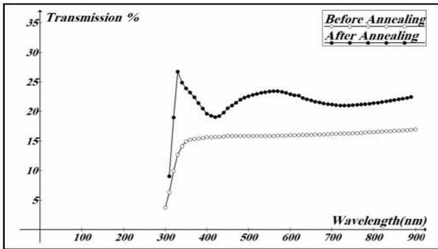
**Figure (2) Transmittance % against Wavelength for (CdO:Ag<sub>2</sub>O) thin films before and after annealing.**
