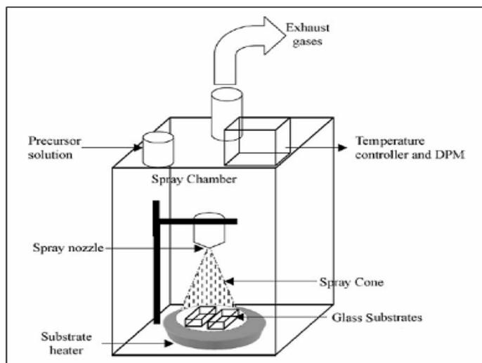
**Figure (1) Spray pyrolysis set-up used for thin film preparation.**
