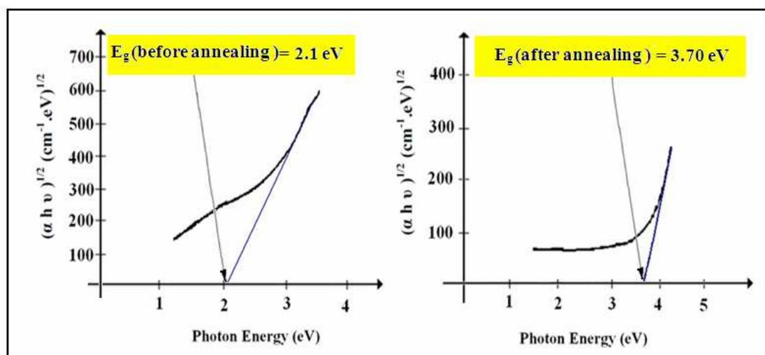
**Figure (4) Optical band gap  $E_g$  estimation for (CdO:Ag<sub>2</sub>O) thin film before and after annealing .**
