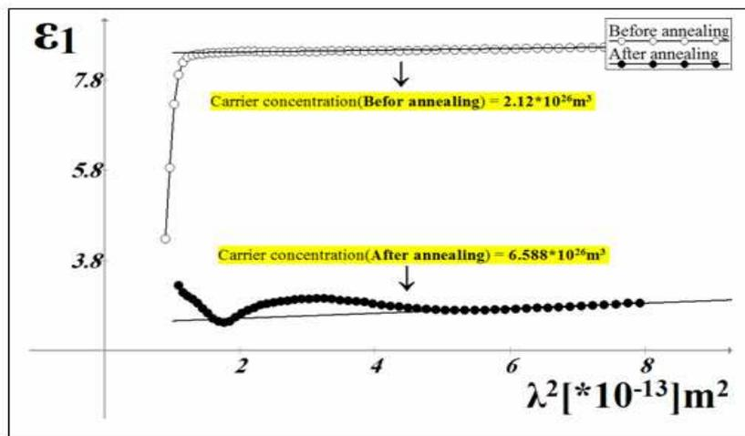
**Figure (7) dielectric constant as a function of  $(\lambda)^2$  for (CdO:Ag<sub>2</sub>O) thin films.**
