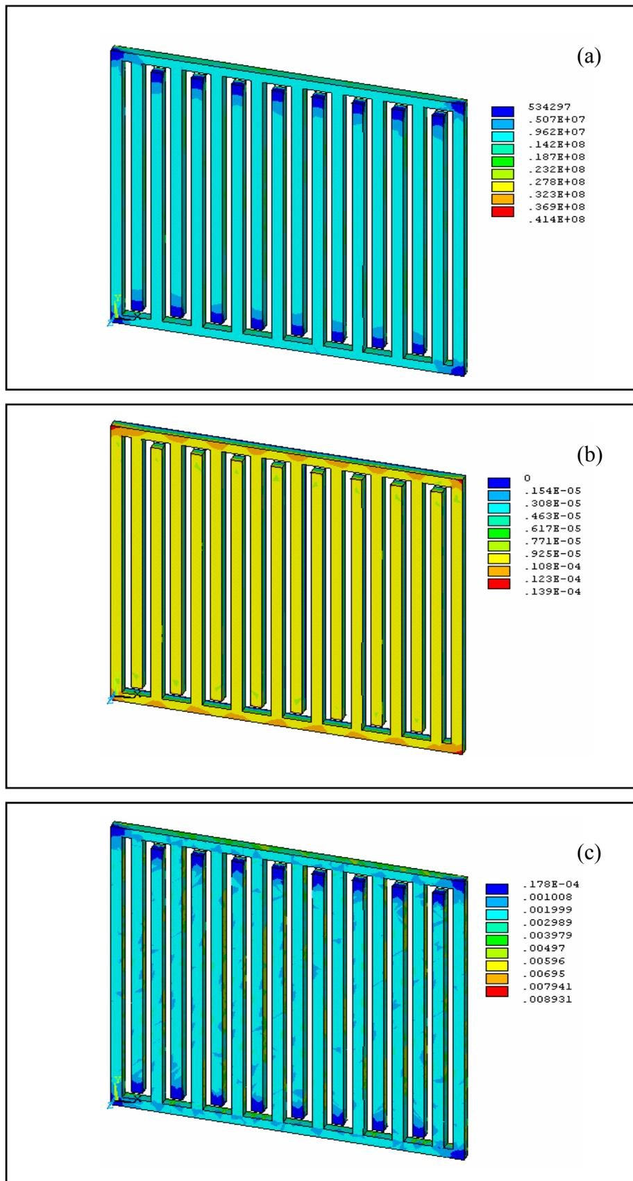
**Fig. 8:** Plate under structural and temperature loads. (a) Stress distribution. (b) Maximum displacement (c) 1<sup>st</sup> principal strain.
