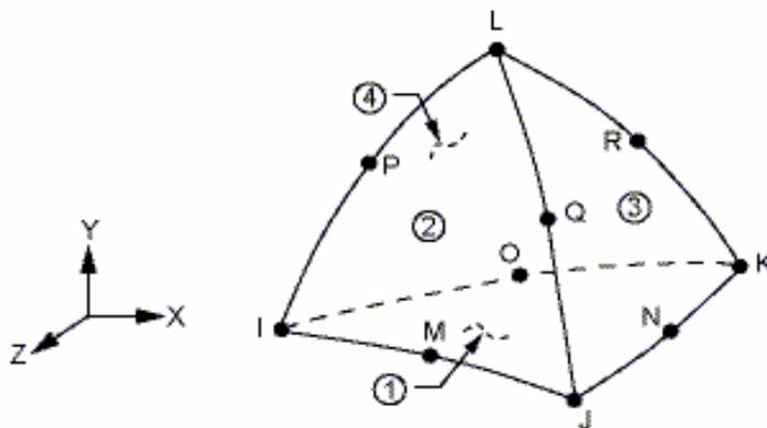
**Fig. 4:** SOLID92 Element (ANSYS Element Reference)
