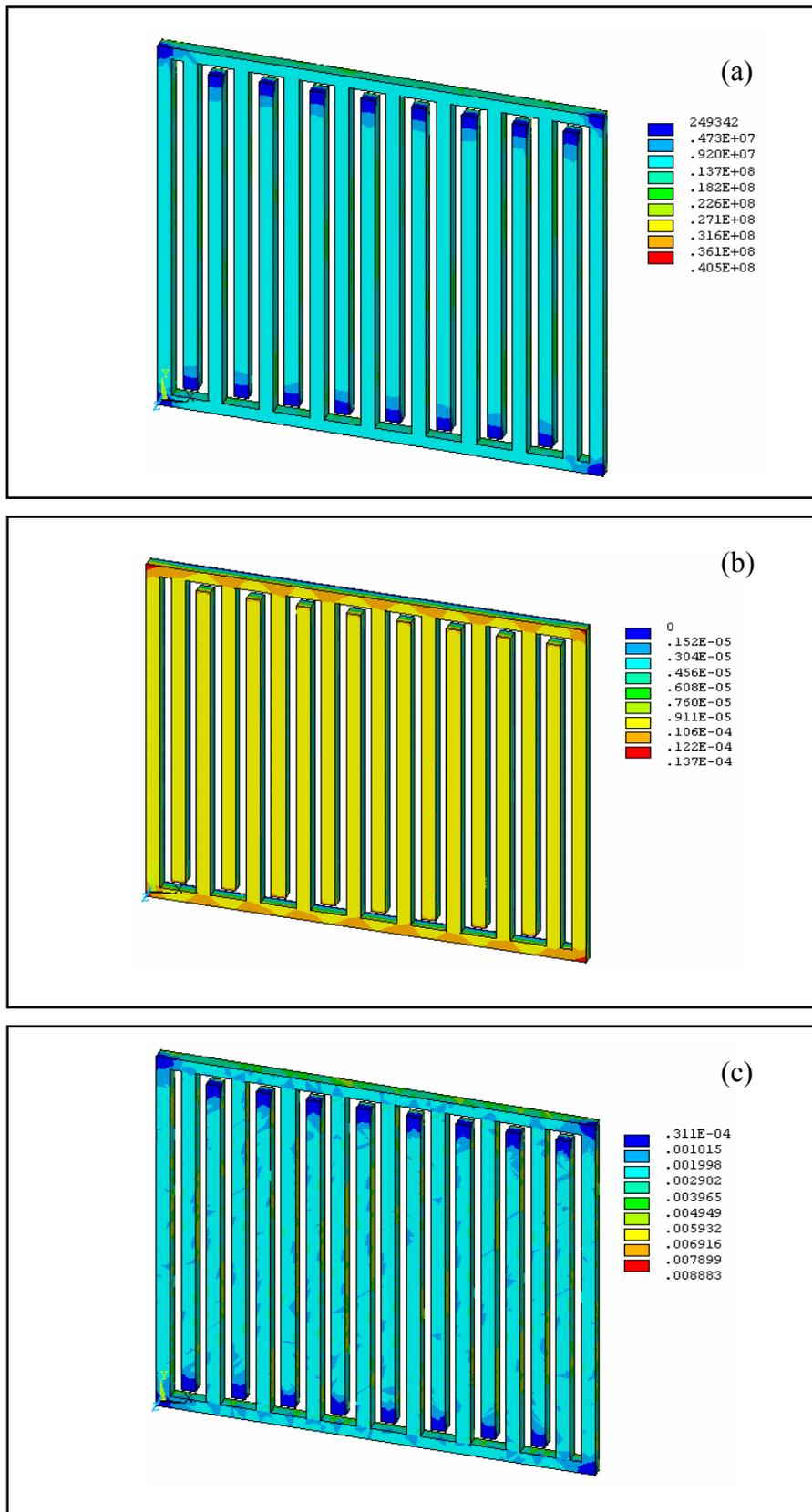
Fig. 7: Plate under temperature load only. (a) Stress distribution. (b) Maximum displacement. (c) 1<sup>st</sup> principal strain.
