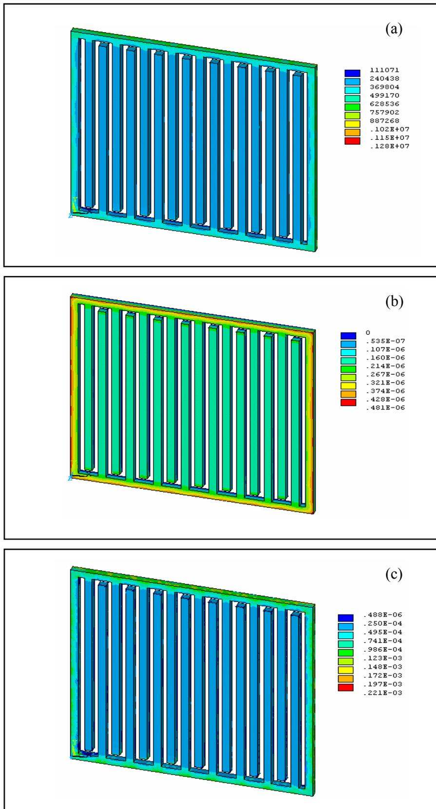
Fig. 6: Plate under pure structural loads. (a) Stress distribution. (b) Maximum displacement. (c) 1<sup>st</sup> principal strain.
