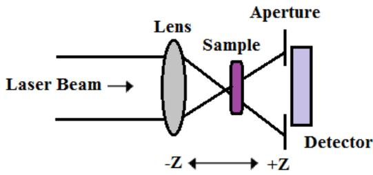
Figure 3 Schematic diagram of experimental arrangement for the Z-scan measurement.
