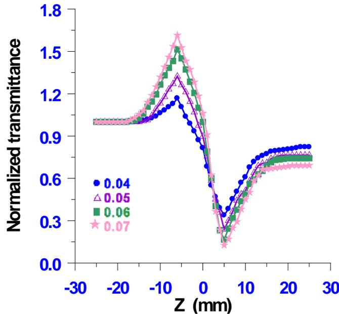
Figure 6 Pure nonlinear refraction curve of dye in solvent at various concentrations.
