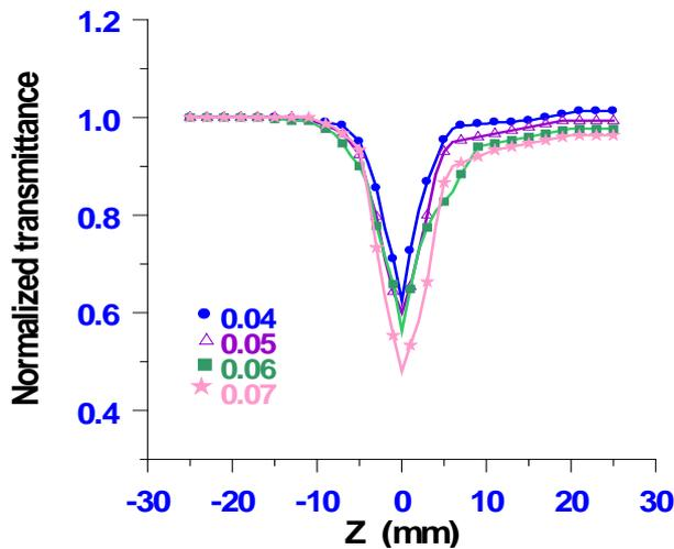
Figure 4 Open-aperture Z-scan data for the THF solution of the azo dye at different concentrations.
