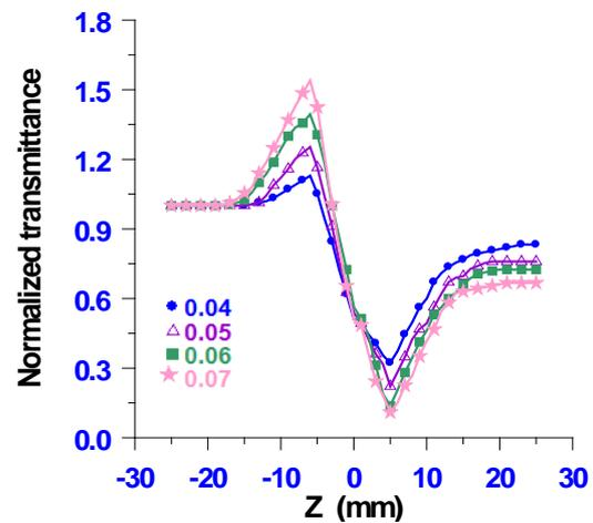
Figure 5 Closed-aperture Z-scan data for the THF solution of the azo dye at different concentrations.
