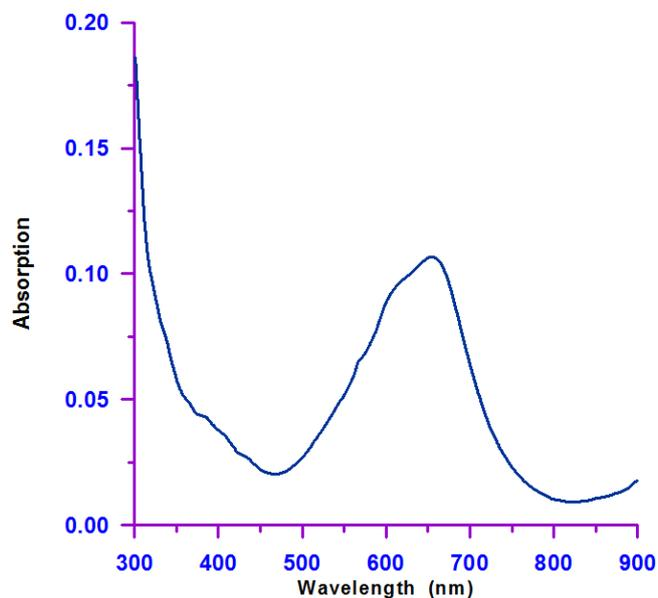
Figure 2 UV-VIS absorption spectrum of janus green dye in tetrahydrofuran solvent.
