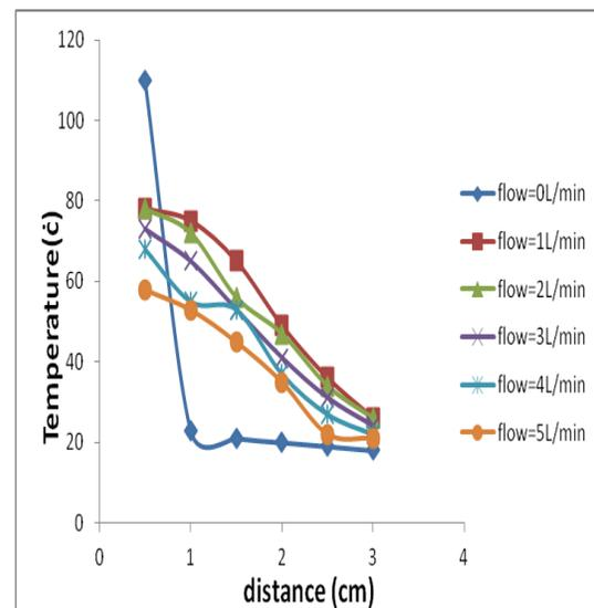
Fig (3): Dependence of the gas temperature on the axial distance between the thermometer and the tip of the needle for various gas flow rates
