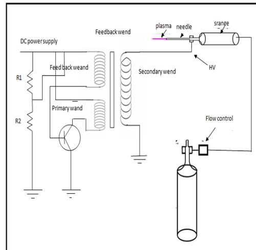
**Fig.(2): Schematic diagram of a non-thermal plasma source**
