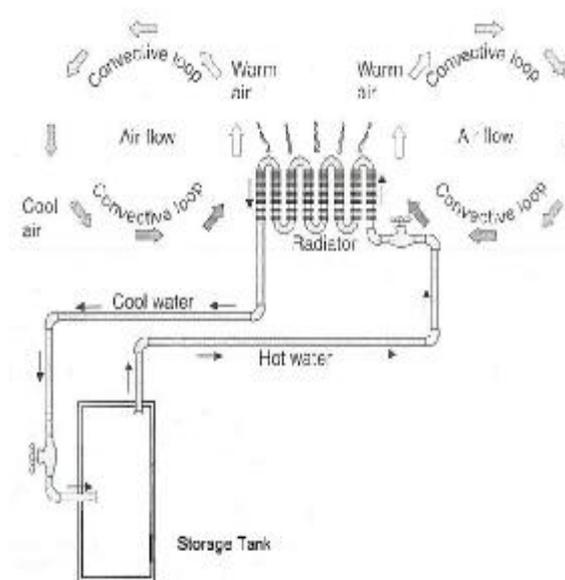
Fig. 4. Convective Loops of Air Flow from Radiator.
