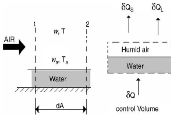
Fig. 6. Schematic Direct Evaporative Cooler.
