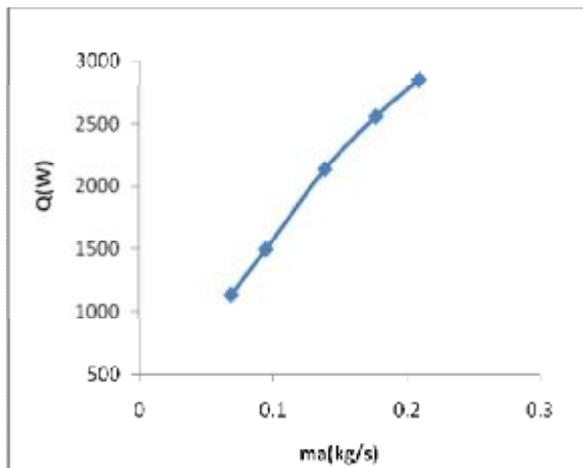
Fig. 9. Variation of Heat Transfer Rate.
