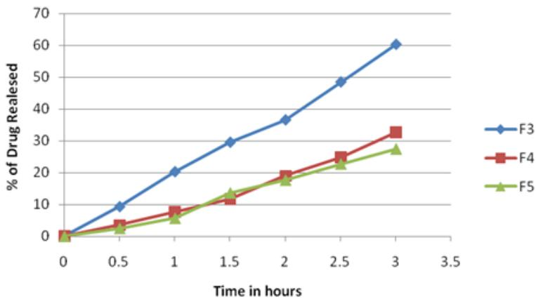
**Figure 3.** Effect of total amount of lipids on in-vitro salbutamol HCl release from liposomal suspension.
