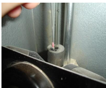
Figure(4): The filled capillary tube was placed inside Electrothermal melting point Apparatus
